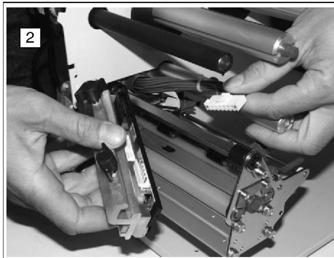
Fig. 7.2.1.b Removing the printhead
