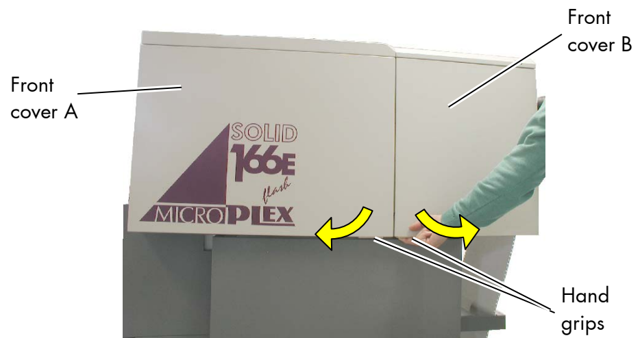
Fig. 6.3.a Opening the front covers
