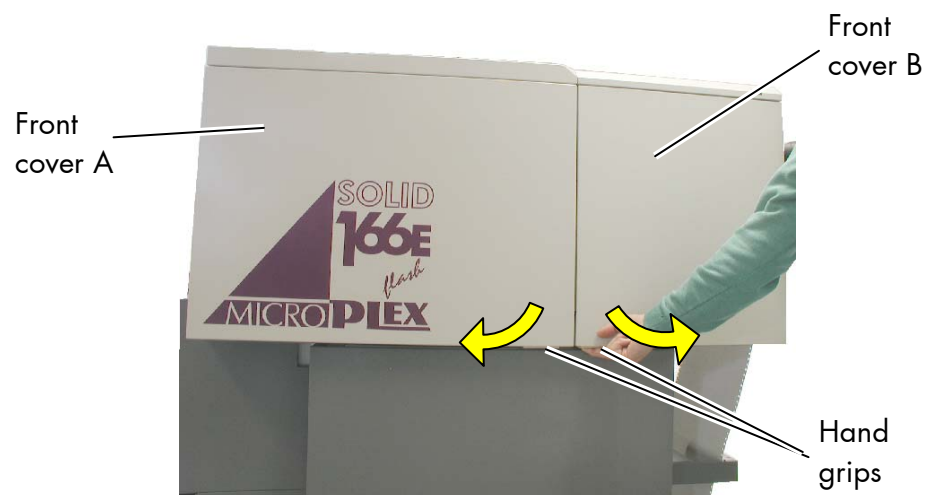
Fig. 6.2.2.a Opening the front covers
