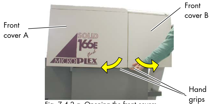
Fig. 7.4.2.a Opening the front covers
