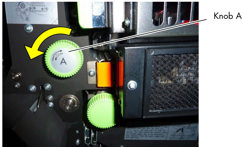
Fig. 7.4.2.k Locking the scuff roller
