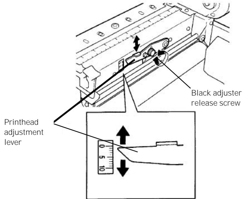
Fig. 5.2.b Adjusting the printhead pressure
