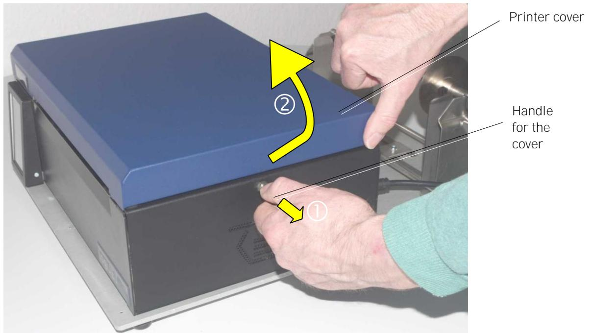
Fig. 2.4.i Opening the printer cover
