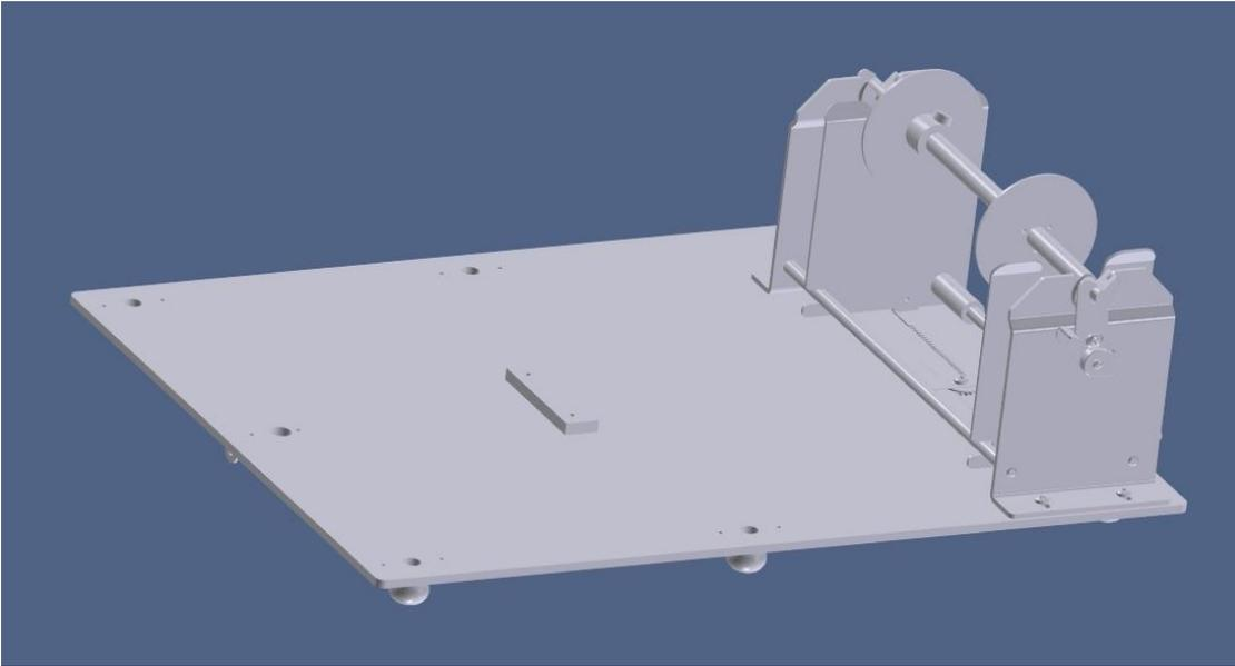
Fig. 2.4.f Mounting Plate for the printer
