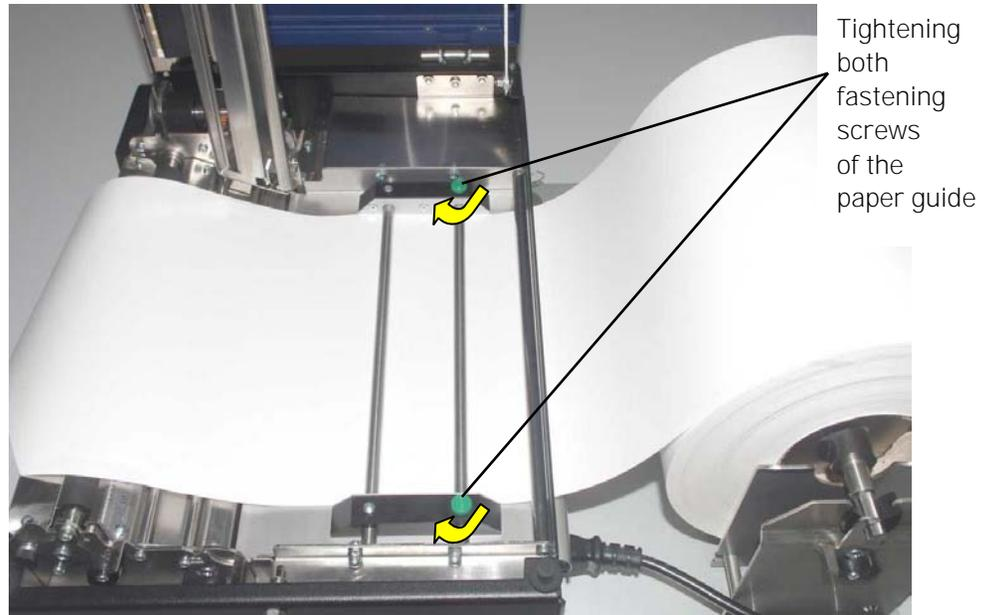
Fig. 5.1.1.r Adjusting the paper guide
