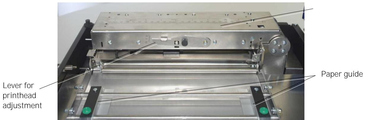
Fig. 2.4.k Details of the printhead
