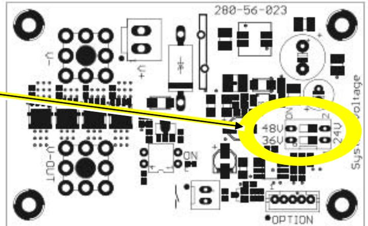
Fig. 6.2.i DIP switch on the DC/DC converter PCB
