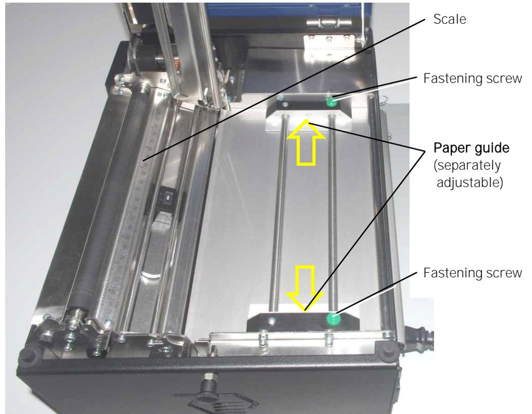
Fig. 5.1.1.h Roughly adjusting the paper guide to new paper width
