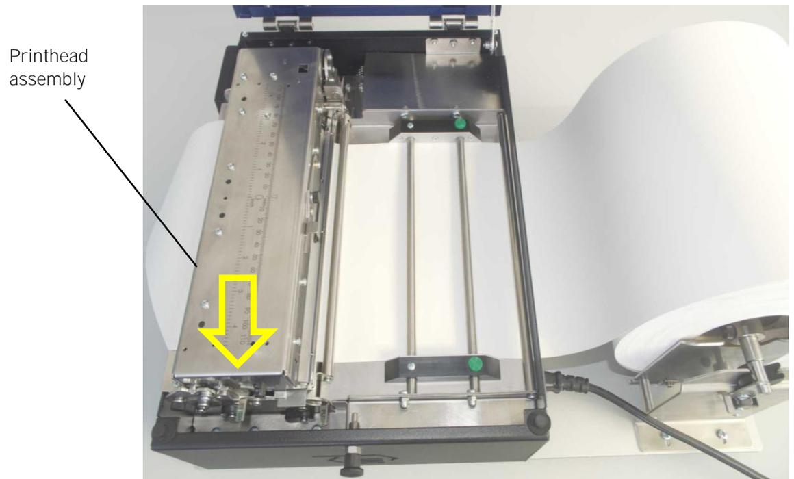
Fig. 5.1.1.u Swivelling down and locking the printhead
