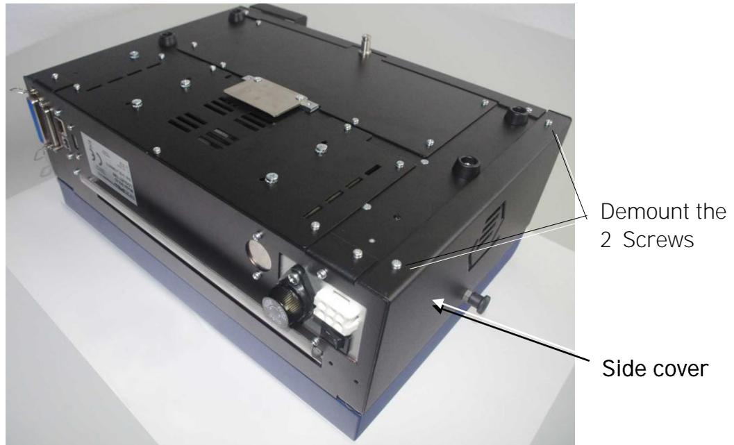
Fig. 6.2.c Underside of the printer: position of the 2 lower screws of the side cover
