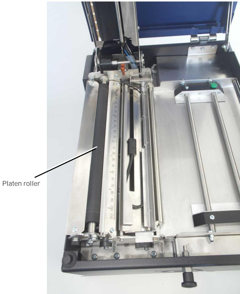
Fig. 10.1.3.b Position of the platen roller
