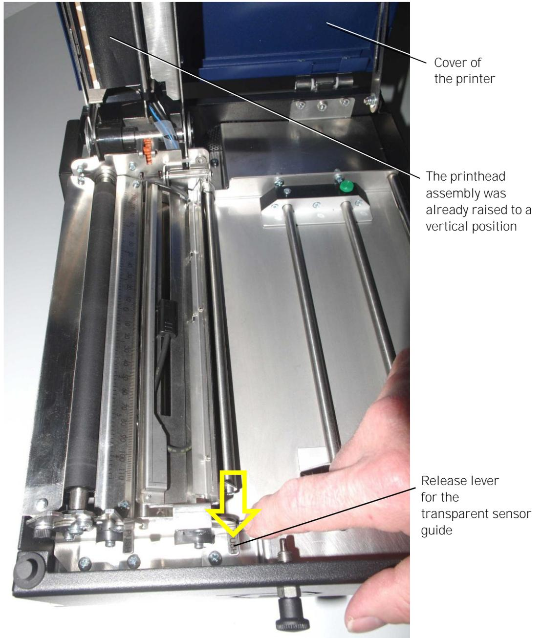
Fig. 10.1.4.a Unlocking the transparent sensor guide
