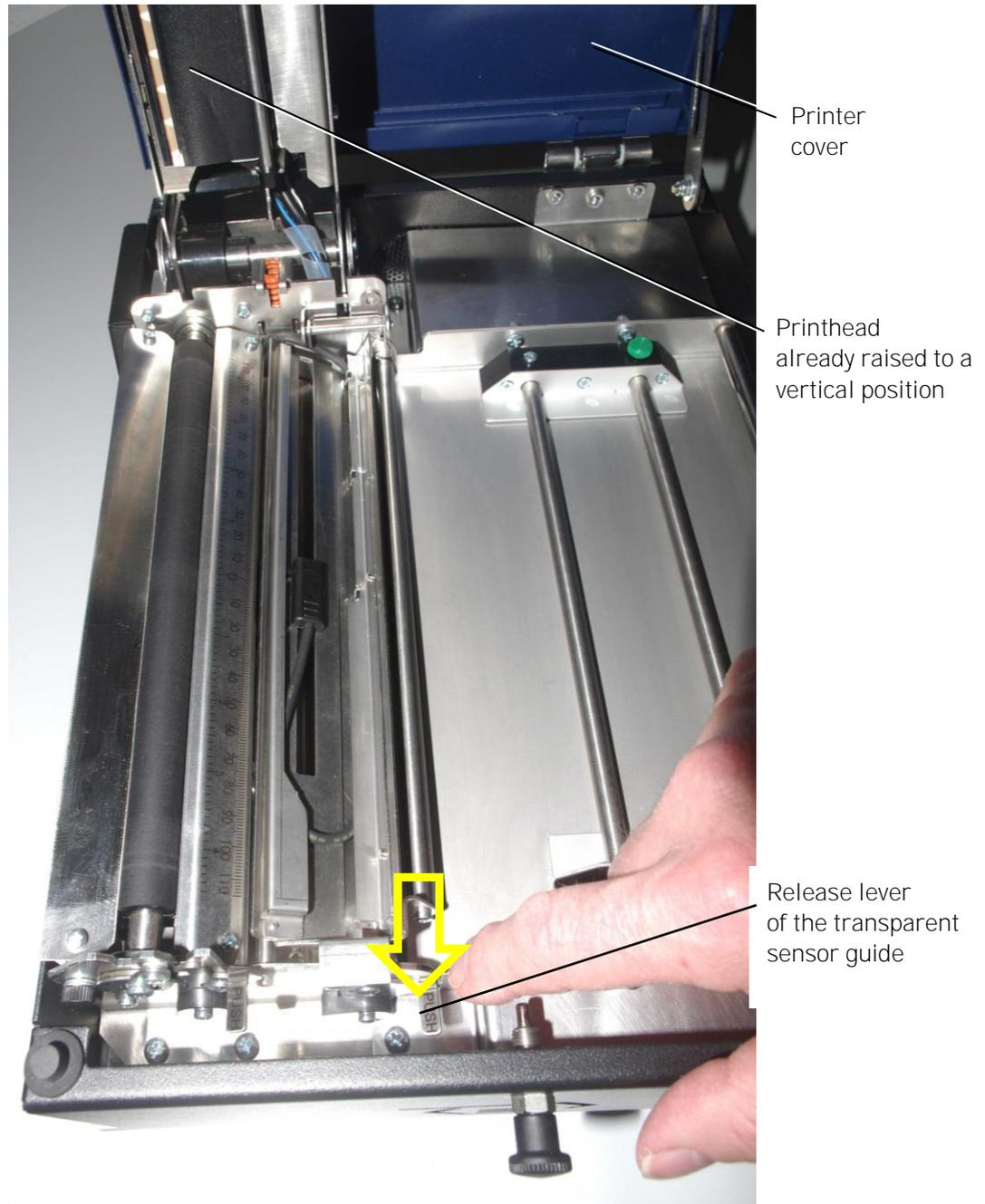
Fig. 5.1.1.f Unlocking the guide of the transparent sensor
