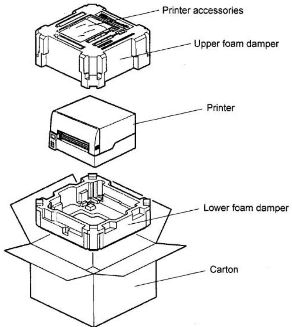
Fig. 2.1.a Example of a Microplex Printer with packing materials
