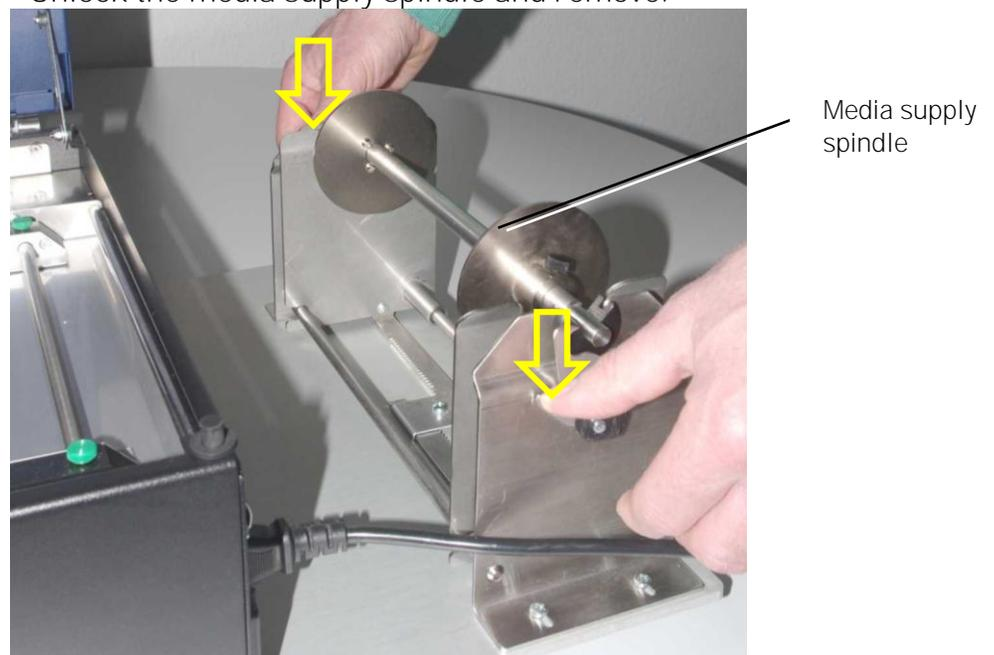
Fig. 5.1.1.i Unlocking and removing the Media supply spindle
