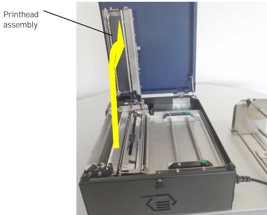
Fig. 9.2.1.d Printhead assembly raised to a vertical position
