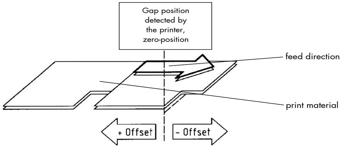
Fig. 9.3.a Setting the zero position of the material feed
