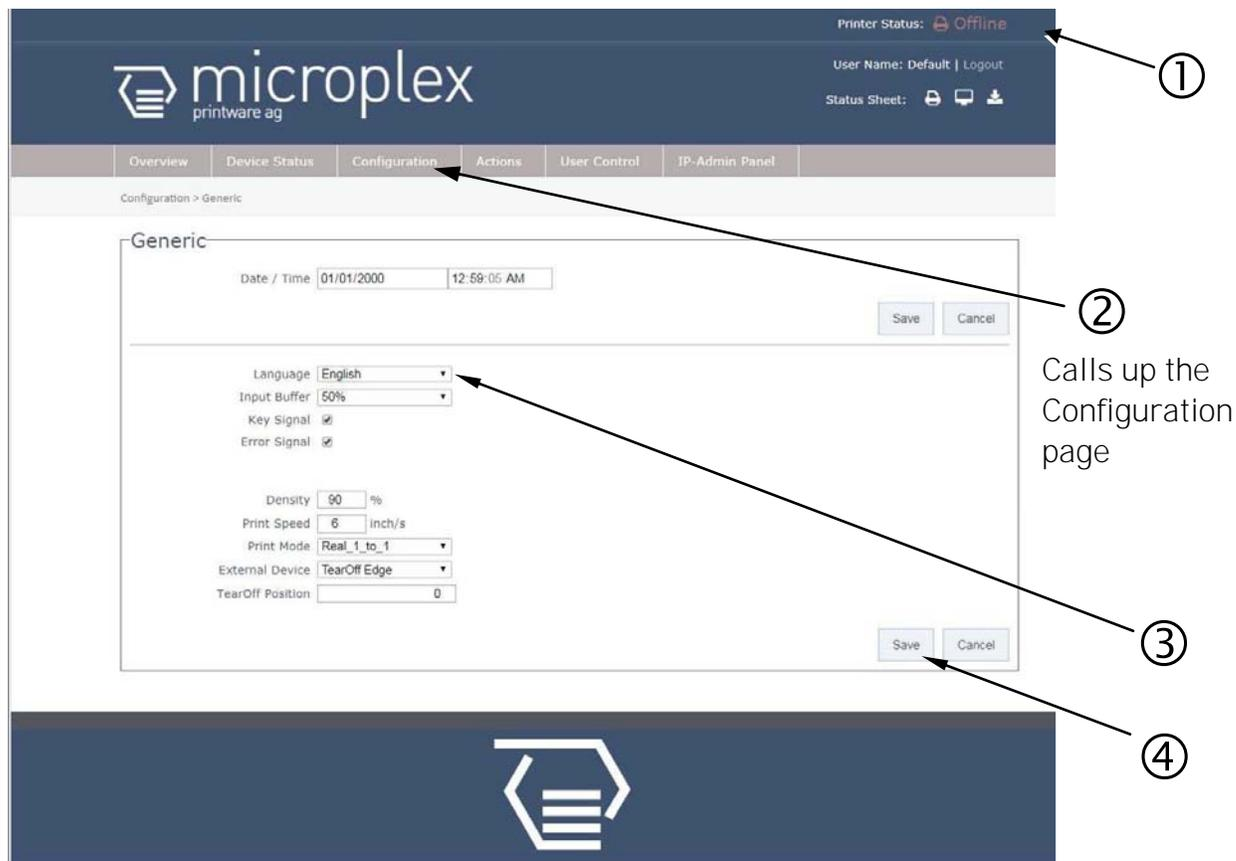
Fig. 7.3.2.a logiJET TM8: Configuration Generic page of the MICROPLEX WebPanel
