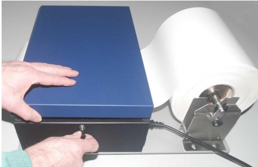
Fig. 11.4.a Opening the cover of the printer
