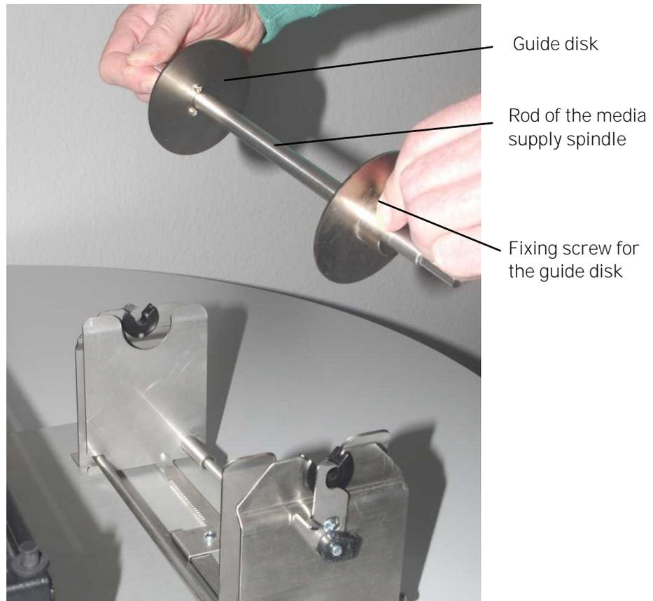
Fig. 5.1.1.j Adjusting both Guide disks of the media supply spindle
