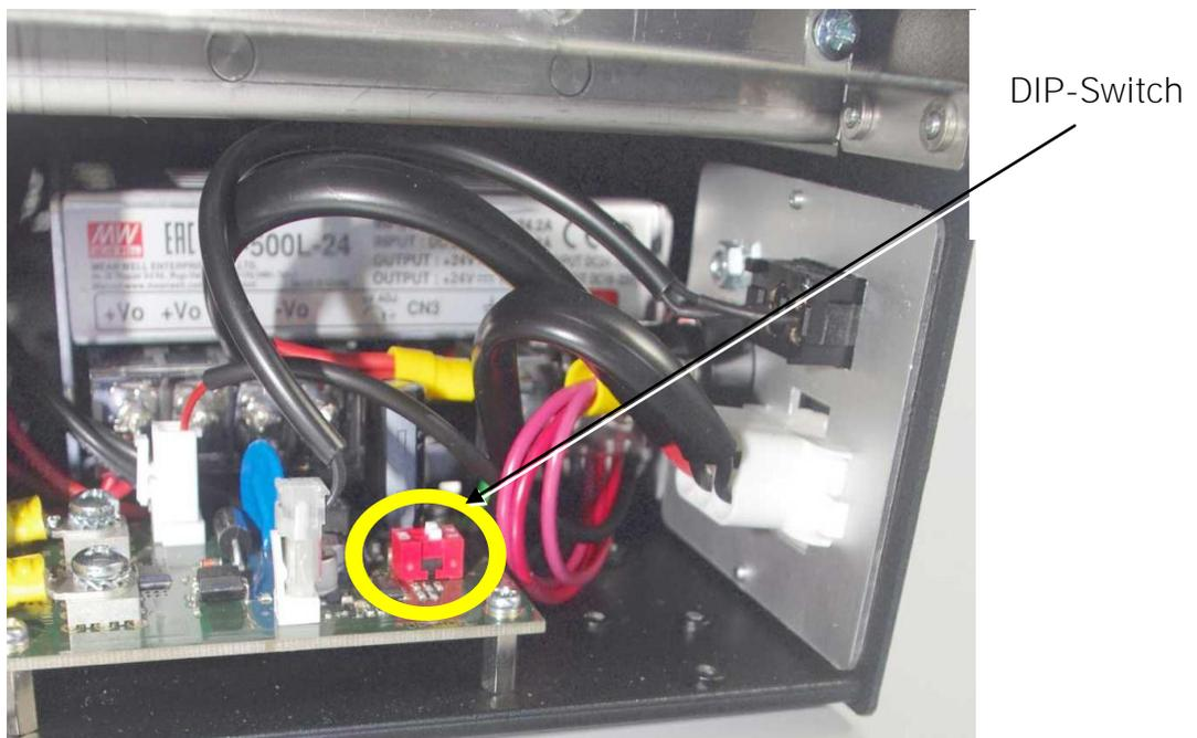
Fig. 6.2.h Close-up view of the DIPswitch
