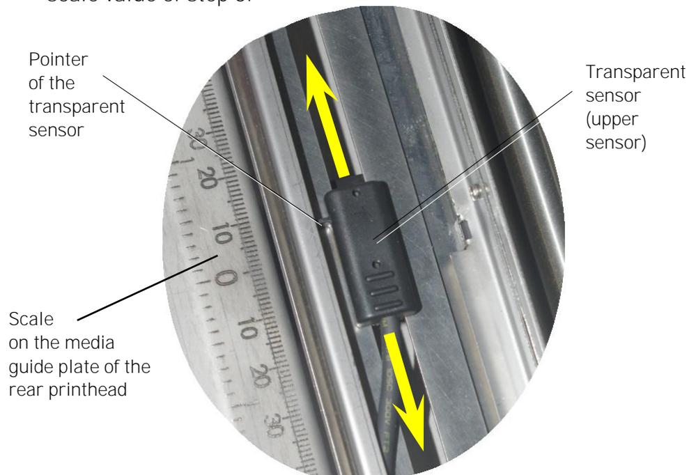
Fig. 9.2.1.i Sliding the **upper sensor** (transparent sensor) to the accurate position
