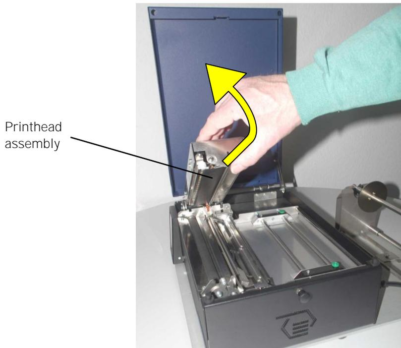
Fig. 5.1.1.d Raising the printhead assembly
