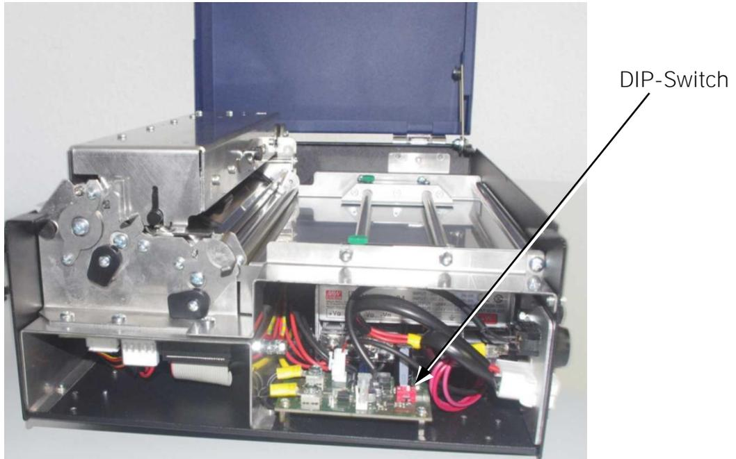
Fig. 6.2.g View inside the printer: Position of the DIPswitch
