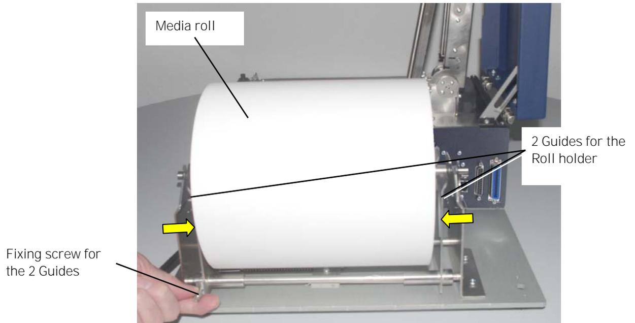
Fig. 5.1.1.n Moving the 2 Guides for the Roll holder towards the Media roll and tightening the fixing screw
