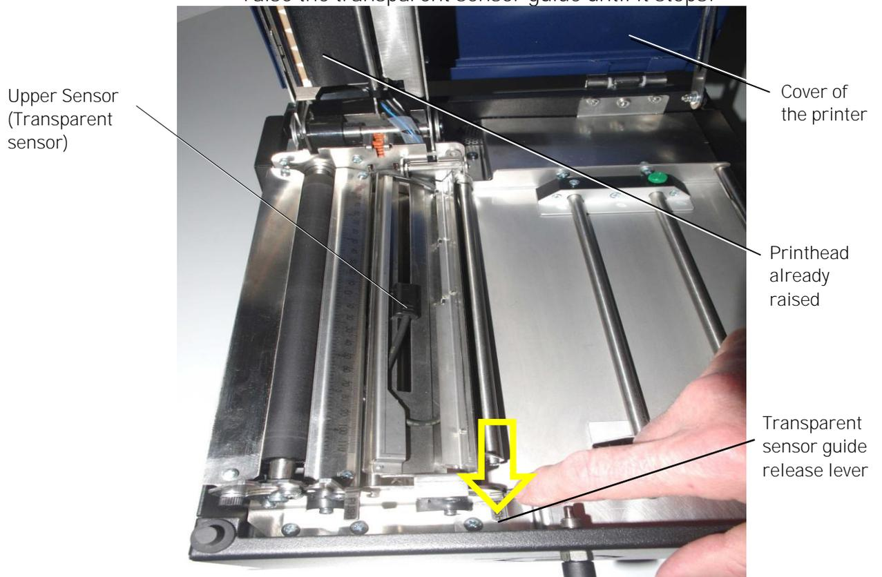
Fig. 9.2.1.e Unlocking the transparent sensor guide
