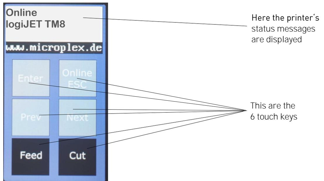
Fig. 6.4.1.a Control Panel of the printer
