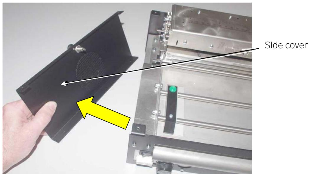
Fig. 6.2.f Remove the side cover of the printer and lay it aside
