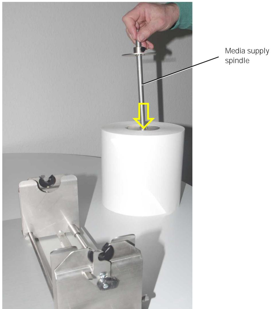
Fig. 5.1.1.k Moving the Media supply spindle into the media roll
