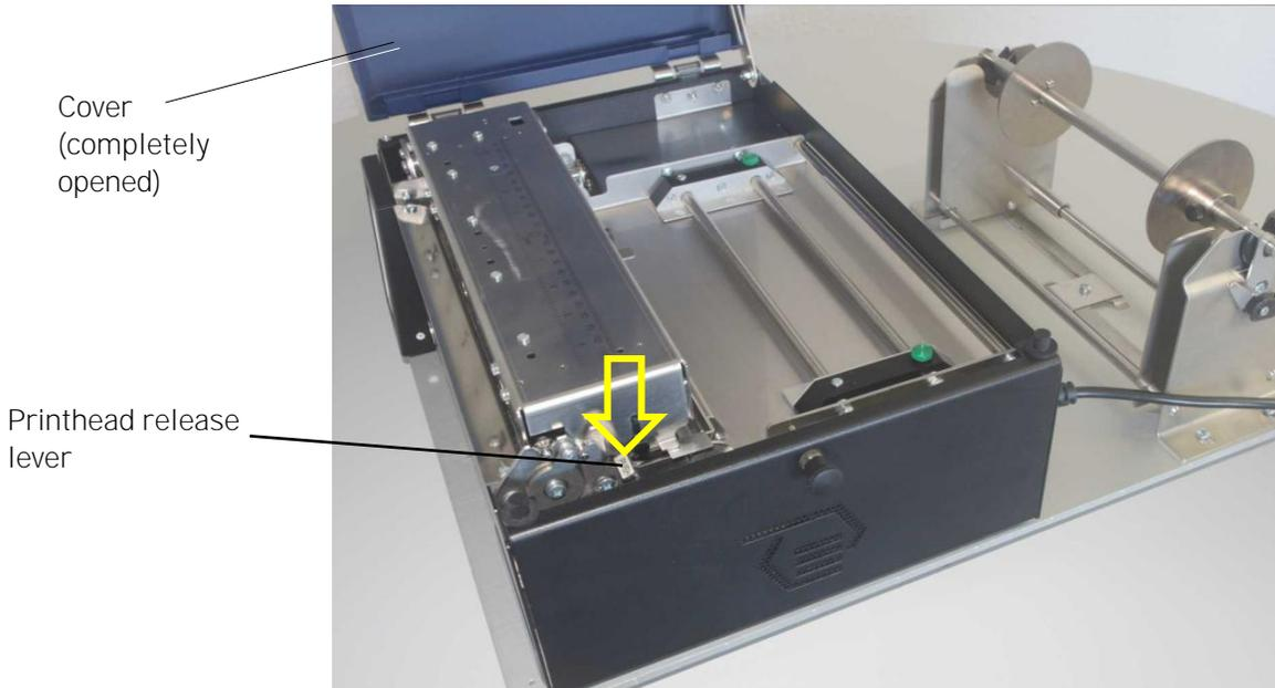
Fig. 9.2.1.b Unlocking the printhead assembly
