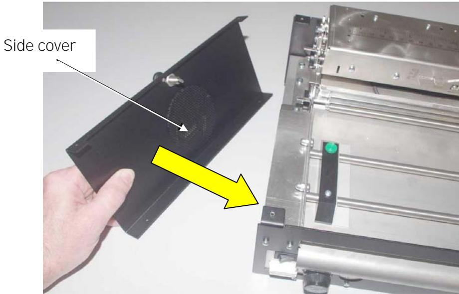
Fig. 6.2.k Take the side cover of the printer
