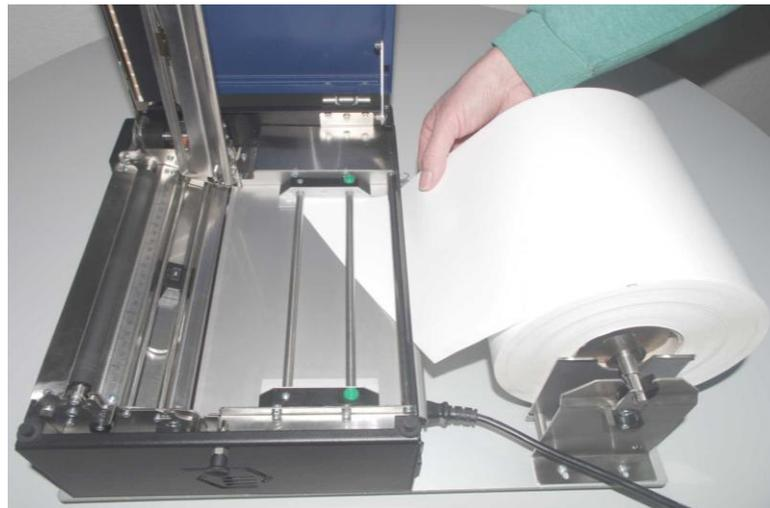
Fig. 5.1.1.o Moving the media into the printer
