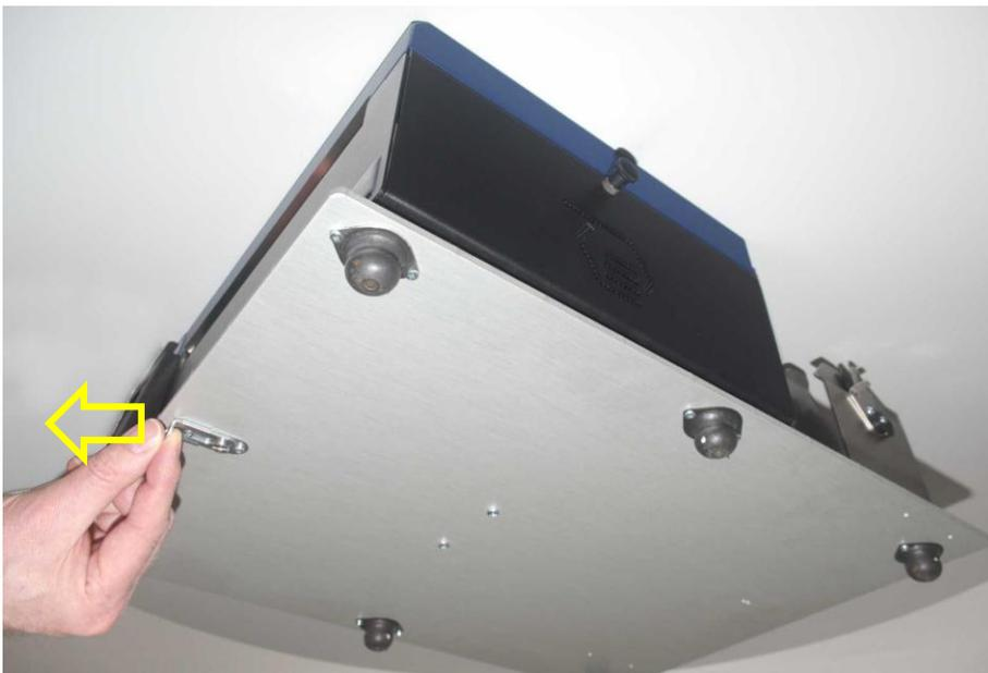
Fig. 2.5.b View from below the printer: Releasing the Mounting Plate
