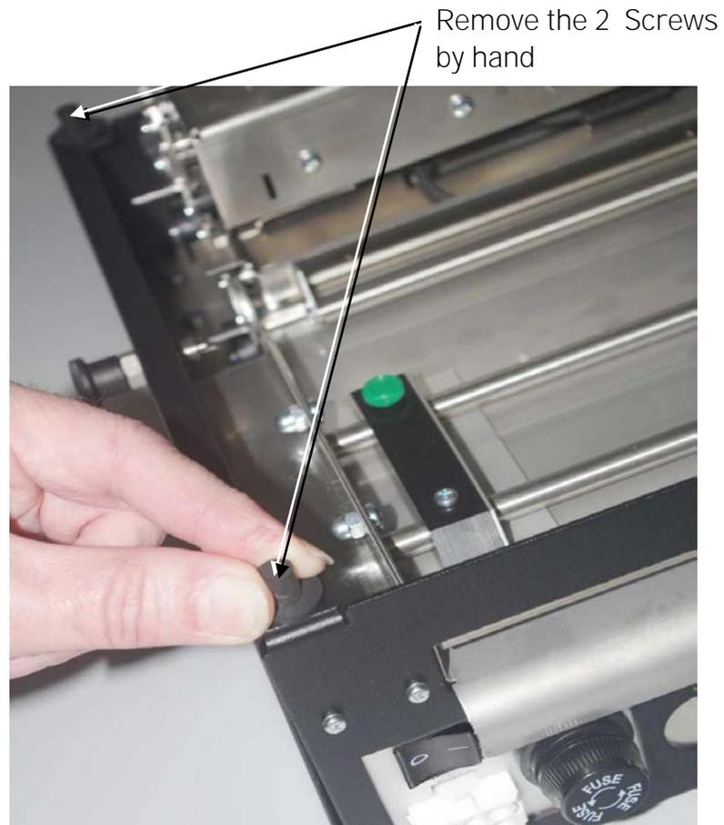
Fig. 6.2.e Remove the 2 upper fastening screws of the side cover
