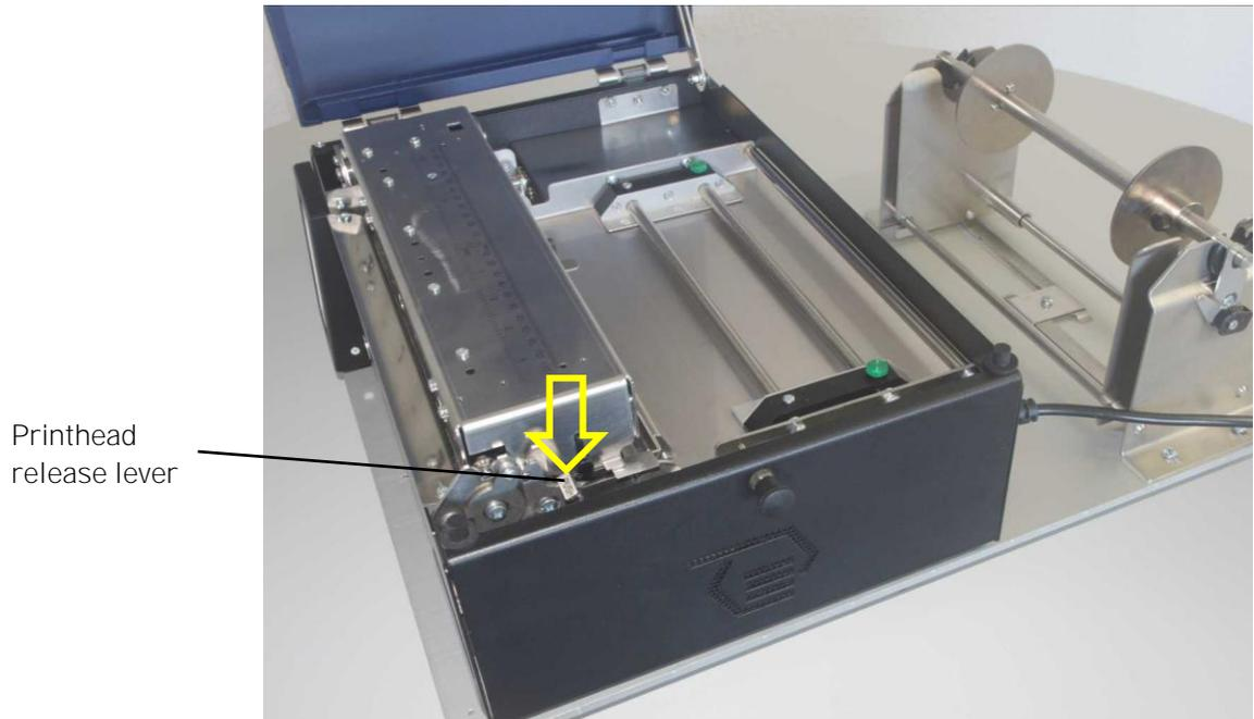
Fig. 10.1.2.b Unlocking the printhead assembly
