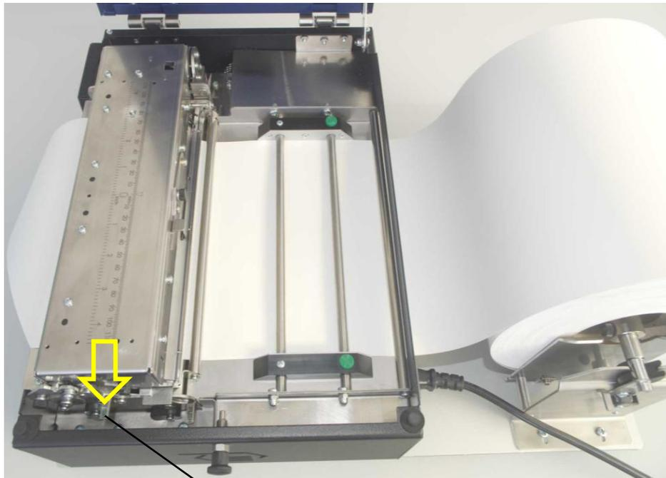
Lever to release the printhead assembly
