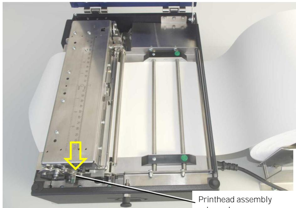
Fig. 11.4.b Releasing the printhead assembly
