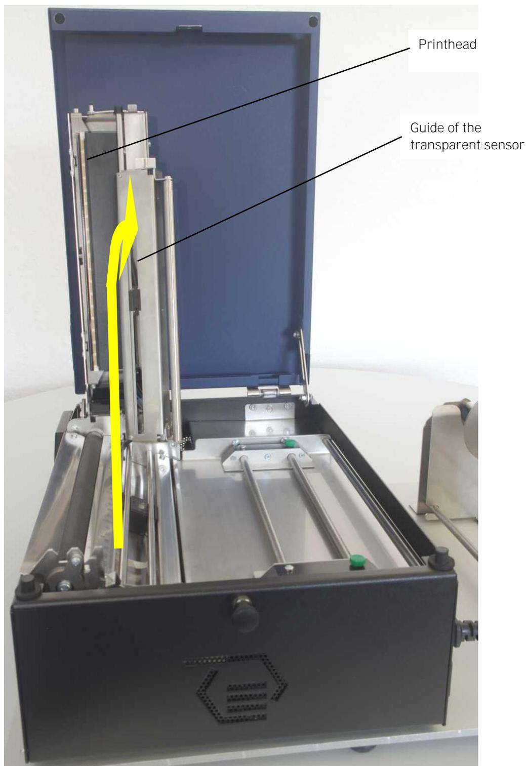
Fig. 5.1.1.g Raising the guide of the transparent sensor
