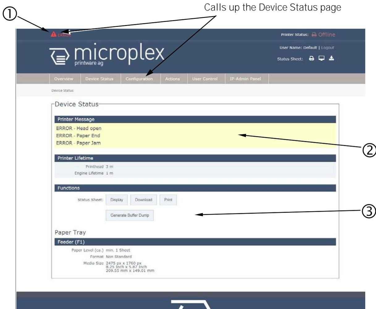
Fig. 7.3.5.a logiJET TM8: Device Status page of the MICROPLEX WebPanel
