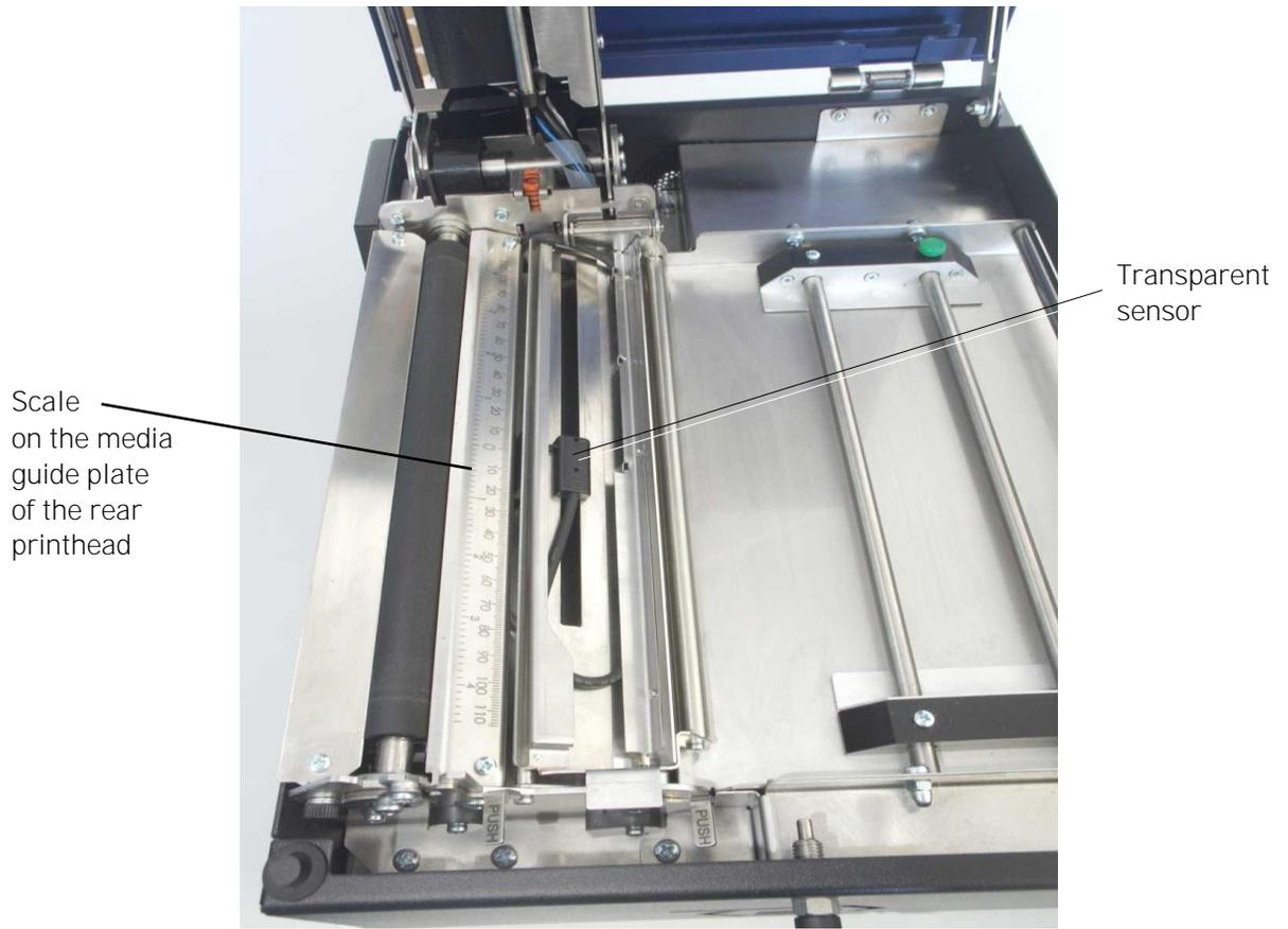
Fig. 9.2.1.h Transparent sensor guide swivelled down
