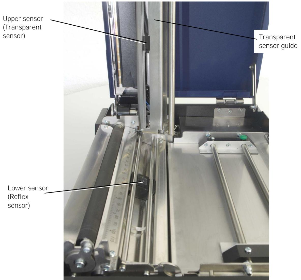
Fig. 10.1.4.c Position of Transparent sensor and Reflex sensor within the printer
