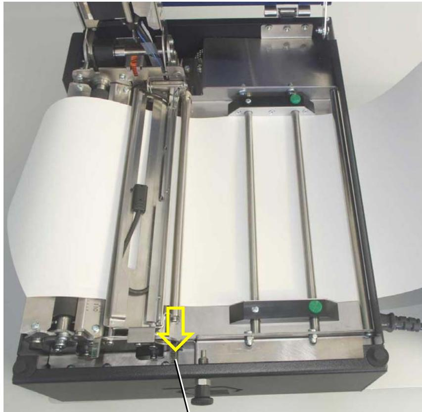
Release lever of the transparent sensor guide
