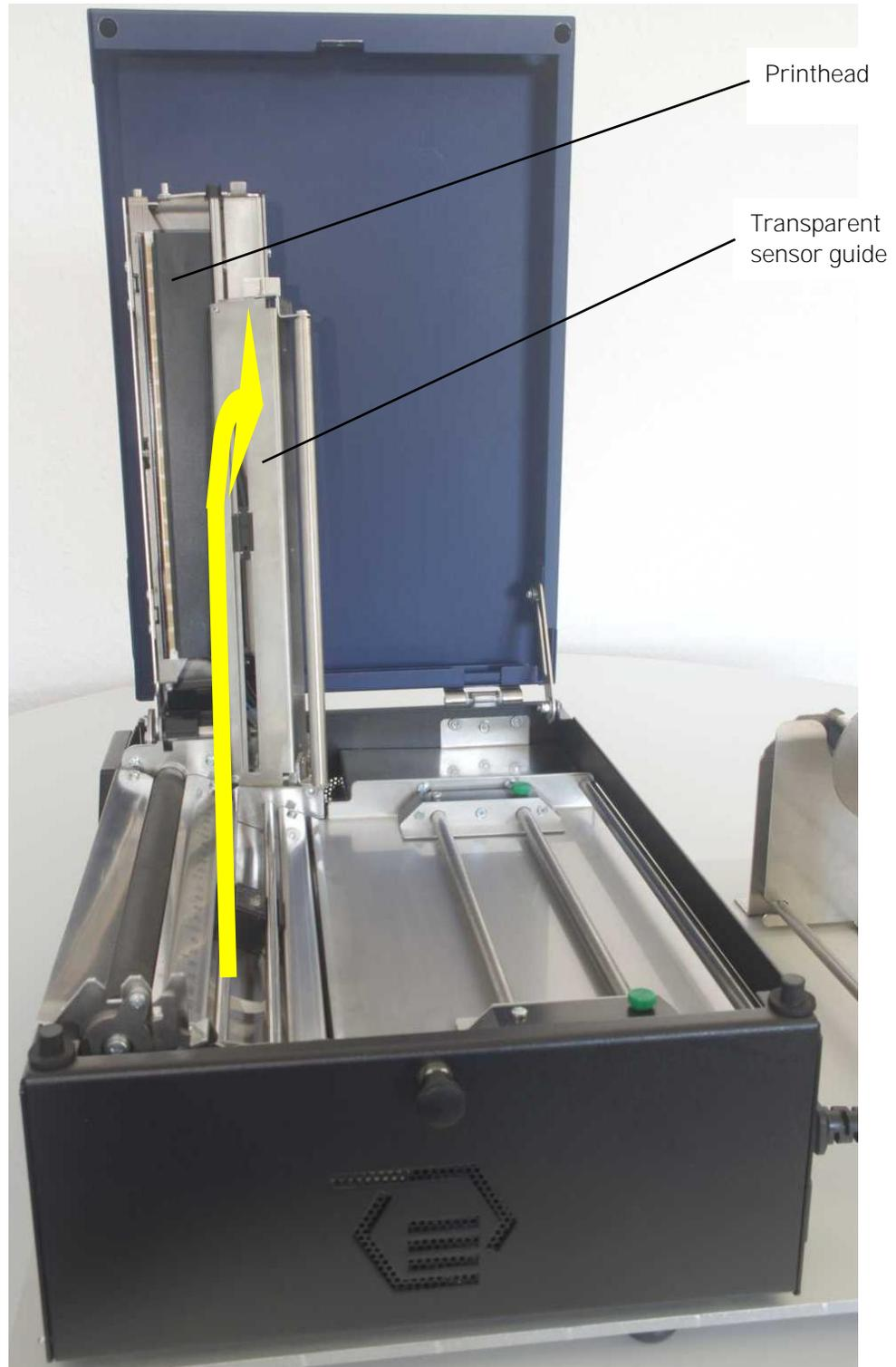
Fig. 10.1.4.b Swivelling the transparent sensor guide upward
