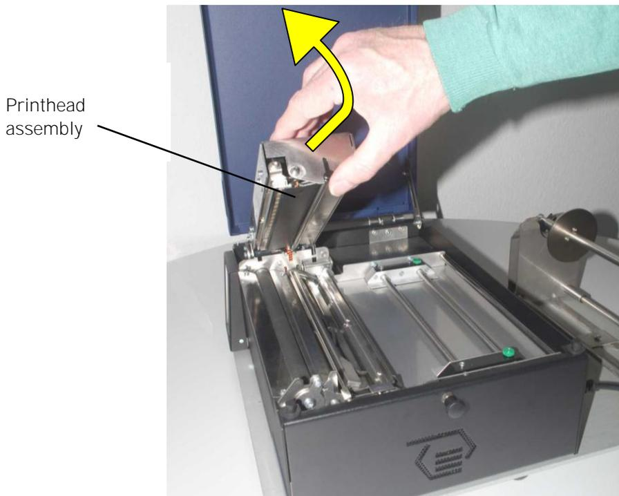
Fig. 9.2.1.c Raising the printhead assembly
