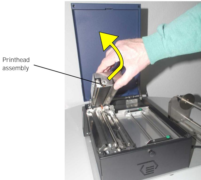
Fig. 10.1.2.c Raising the printhead assembly
