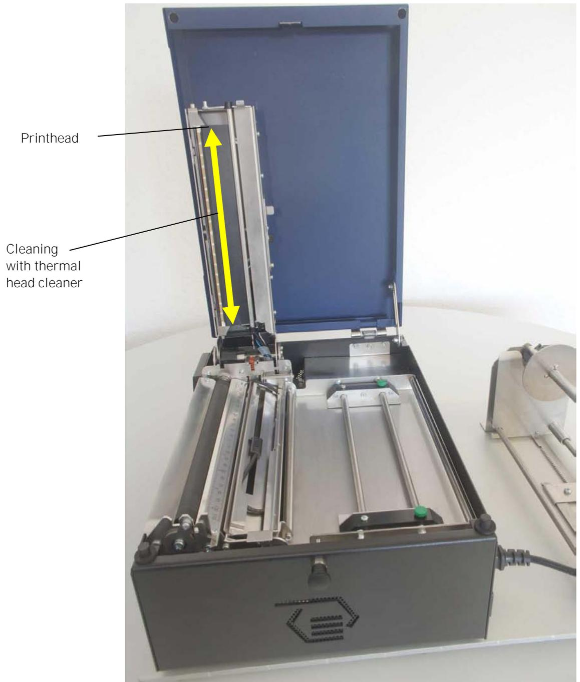
Fig. 10.1.2.d Cleaning the printhead
