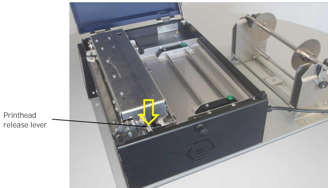
Fig. 10.1.3.a Unlocking the printhead assembly
