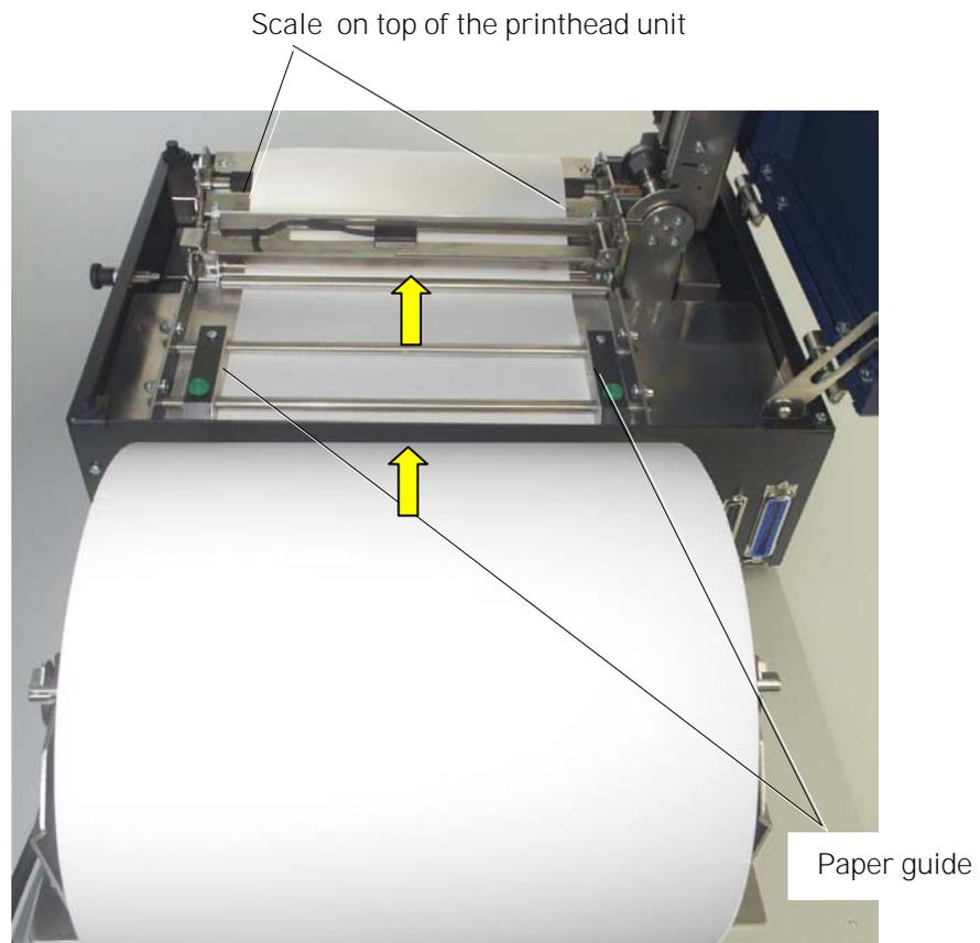
Fig. 5.1.1.t Checking the straight course of the media
