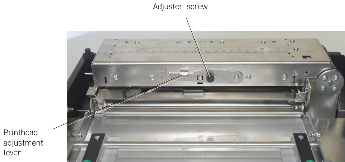
Fig. 5.2.a The black Adjuster screw has to be loosen for adjustments
