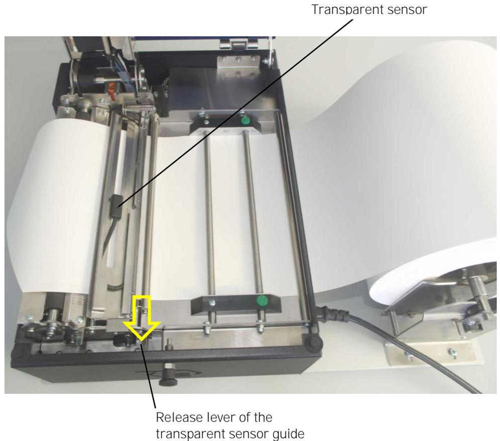
Fig. 5.1.2.b Unlocking the transparent sensor guide (in order to raise it)
