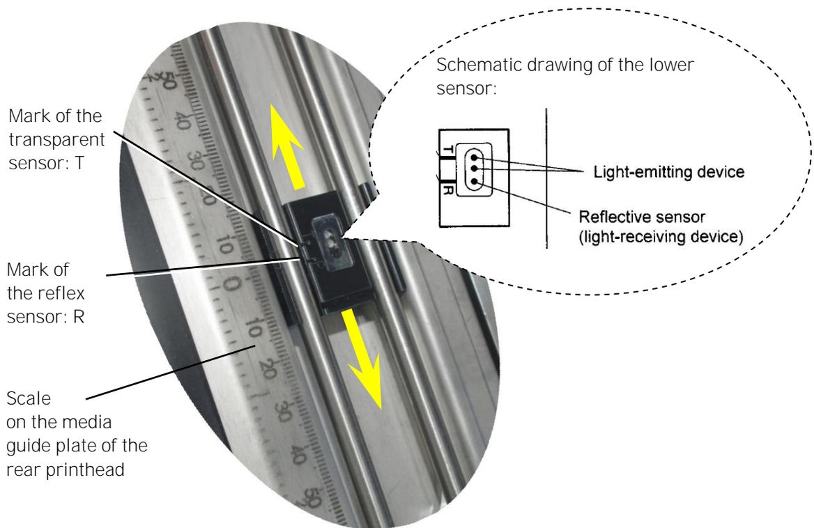
Fig. 9.2.1.g Setting **the lower** sensor to the right position
