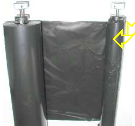
Fig. 5.2.2.f Winding the end of the ribbon
