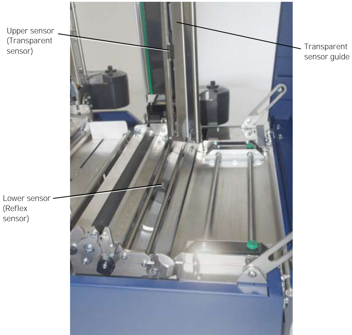
Fig. 8.1.4.c Position of Transparent sensor and Reflex sensor within the printer
