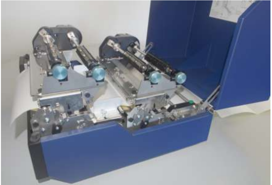
Fig. 5.1.1.m Both printhead assemblies are swivelled down and locked
