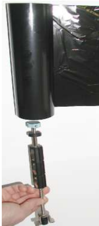
Fig. 5.2.2.c Inserting the ribbon mandrels into the ribbon roll and into the ribbon takeup core
