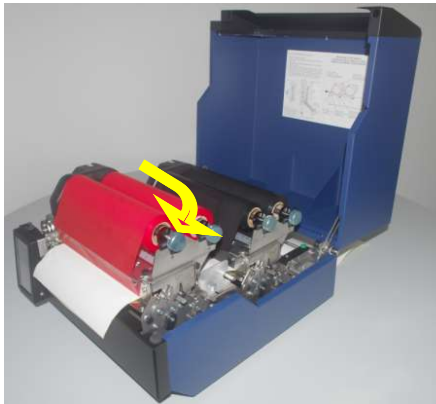
Fig. 5.2.2.k Printer with ribbons installed
