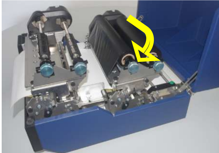
Fig. 5.2.2.j Swivelling the rear printhead assembly downward and locking it
