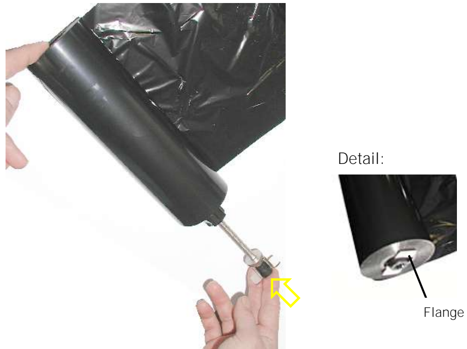
Fig. 5.2.2.d Sliding the ribbon mandrel completely into the ribbon roll
