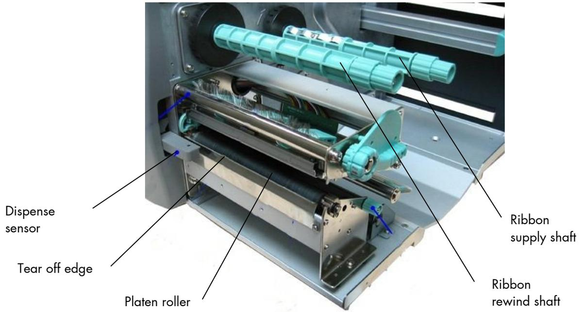
Fig. 2.4.d Details printer mechanism
