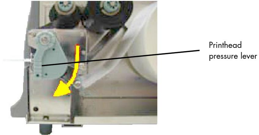
Fig. 5.4.e Locking the pressure lever
