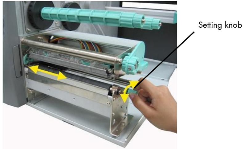
Fig. 5.2.1.k Adjusting the sensor position
