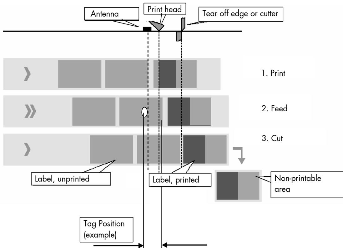
**Hints:** In the RFID mode a tear off (single label operation) is useful only on condition that the distance between the transponder and the beginning of the label is greater than 31 mm (Tag Position). (See section 10.2.1 Selecting the RFID Mode and 10.2.3 Adjusting the Transponder Position as well as the comments in figure 10.4.1.a).
