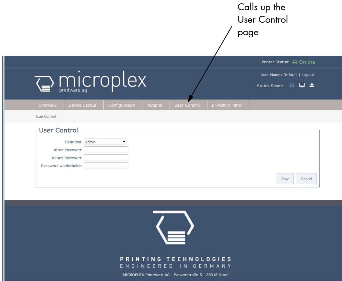
Fig. 7.3.7.a logiJET T4-2 /T6-2: User Control page of the MICROPLEX WebPanel
