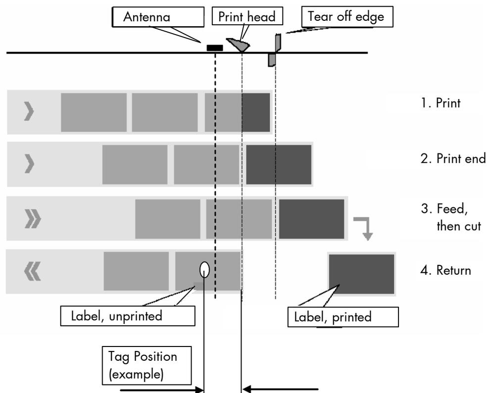
**Hints:** In the RFID mode a tear off (single label operation) is useful only on condition that the distance between the transponder and the beginning of the label is greater than 31 mm (Tag Position). (See section 10.2.1 Selecting the RFID Mode and 10.2.3 Adjusting the Transponder Position as well as the comments in figure 10.4.1.a).
