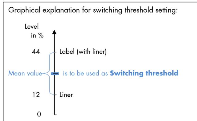
The **middle between the label level** (incl. liner) **and the liner level** has to be calculated:
