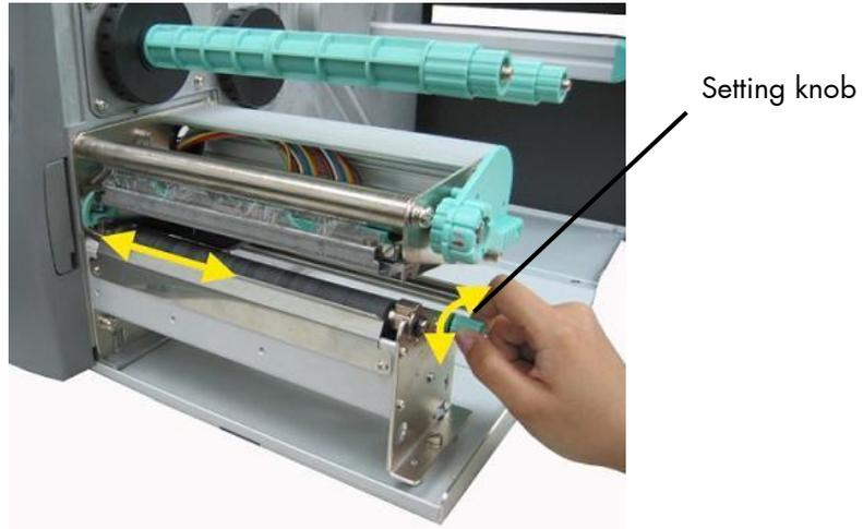
Fig. 9.3.1.d Adjusting the sensor position
