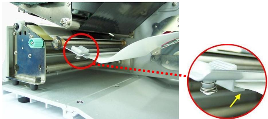
Fig. 5.2.1.j Setting the material guide
