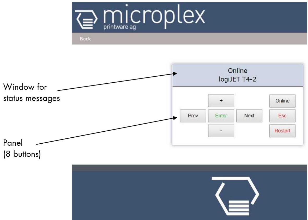
Fig. 7.4.2.a MICROPLEX IP-Panel (virtual control panel of the logiJET T4-2 /T6-2)
