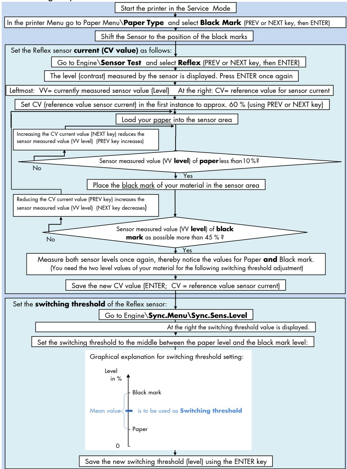
Description of the Working Steps for the **Reflex Sensor** (Black Mark Sensor):
