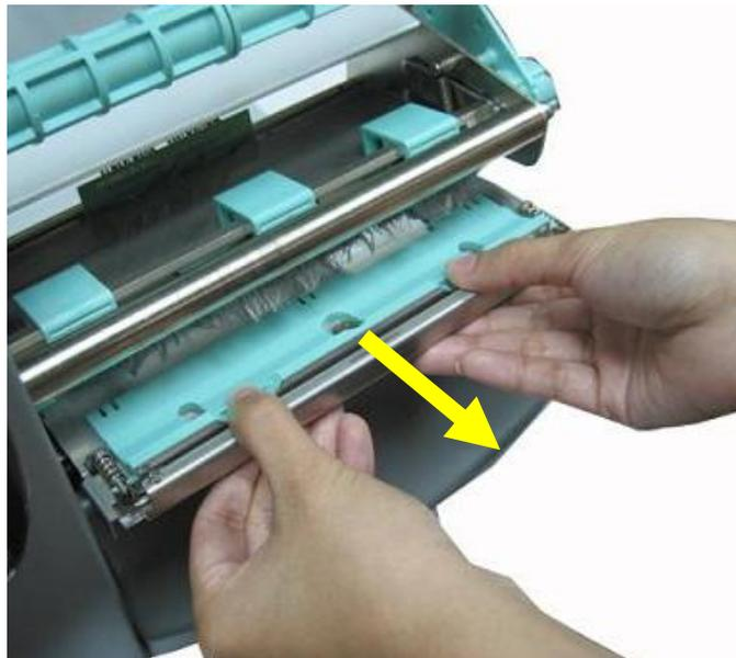
Fig. 11.2.1.c Removing the printhead
