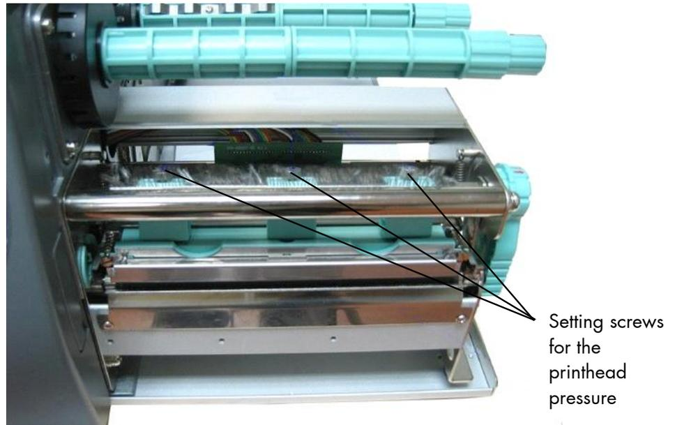
Fig. 5.4.f Adjusting the printhead's contact pressure
