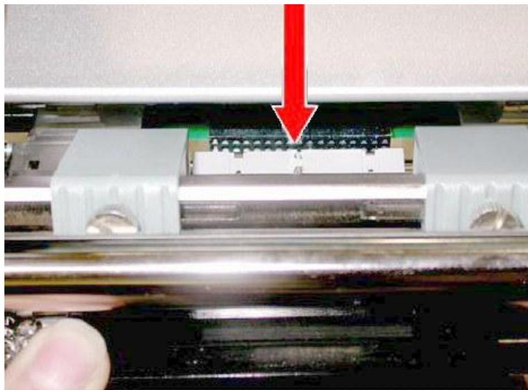
Fig. 11.2.1.e Line up the printhead plug
