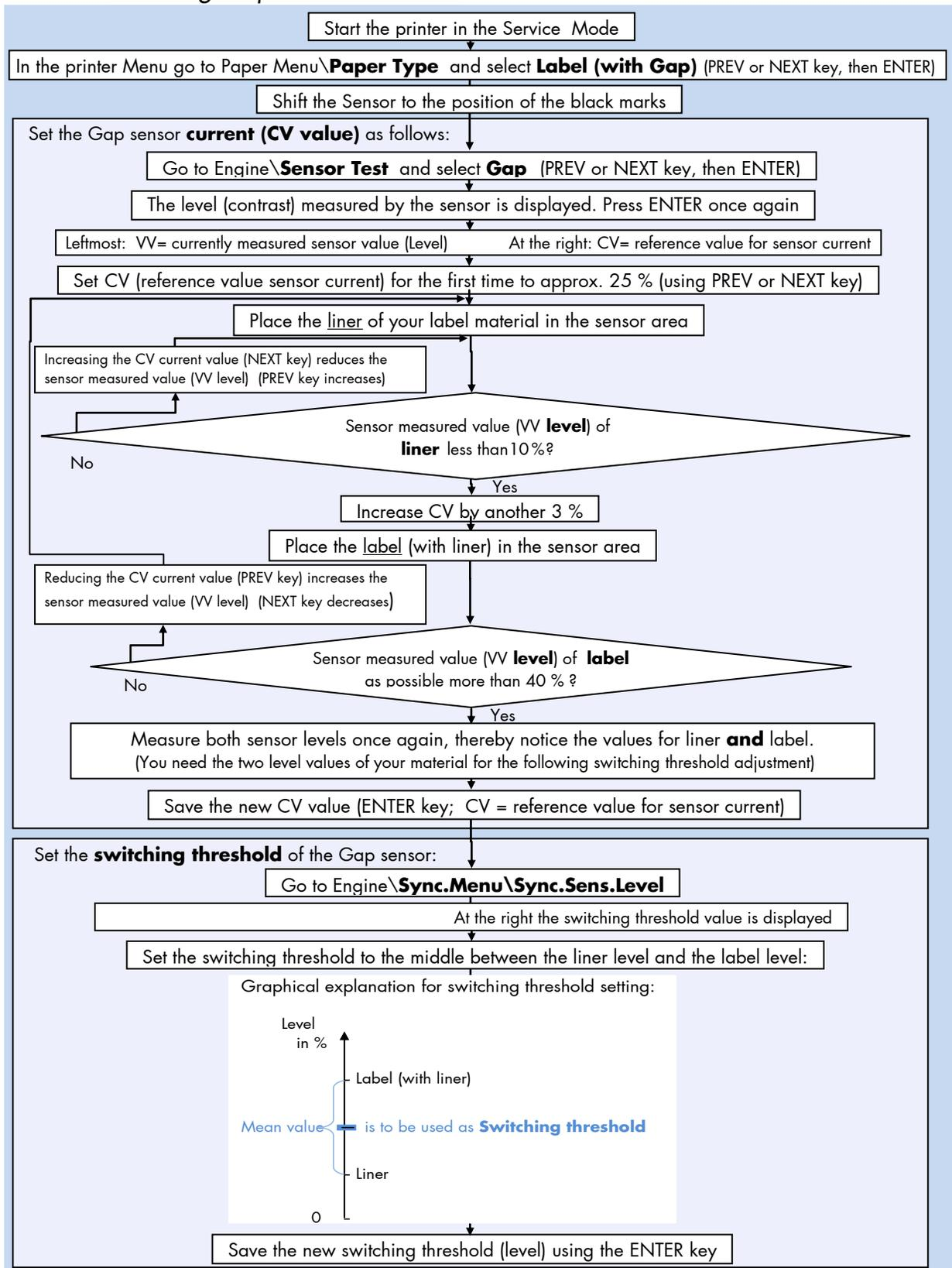
Description of the Working Steps for the **Gap Sensor** (Transparent Sensor):
