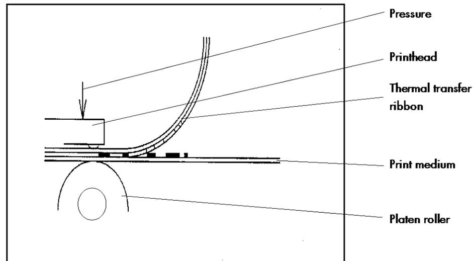
Fig. 11.3.a Principle view of the print process
