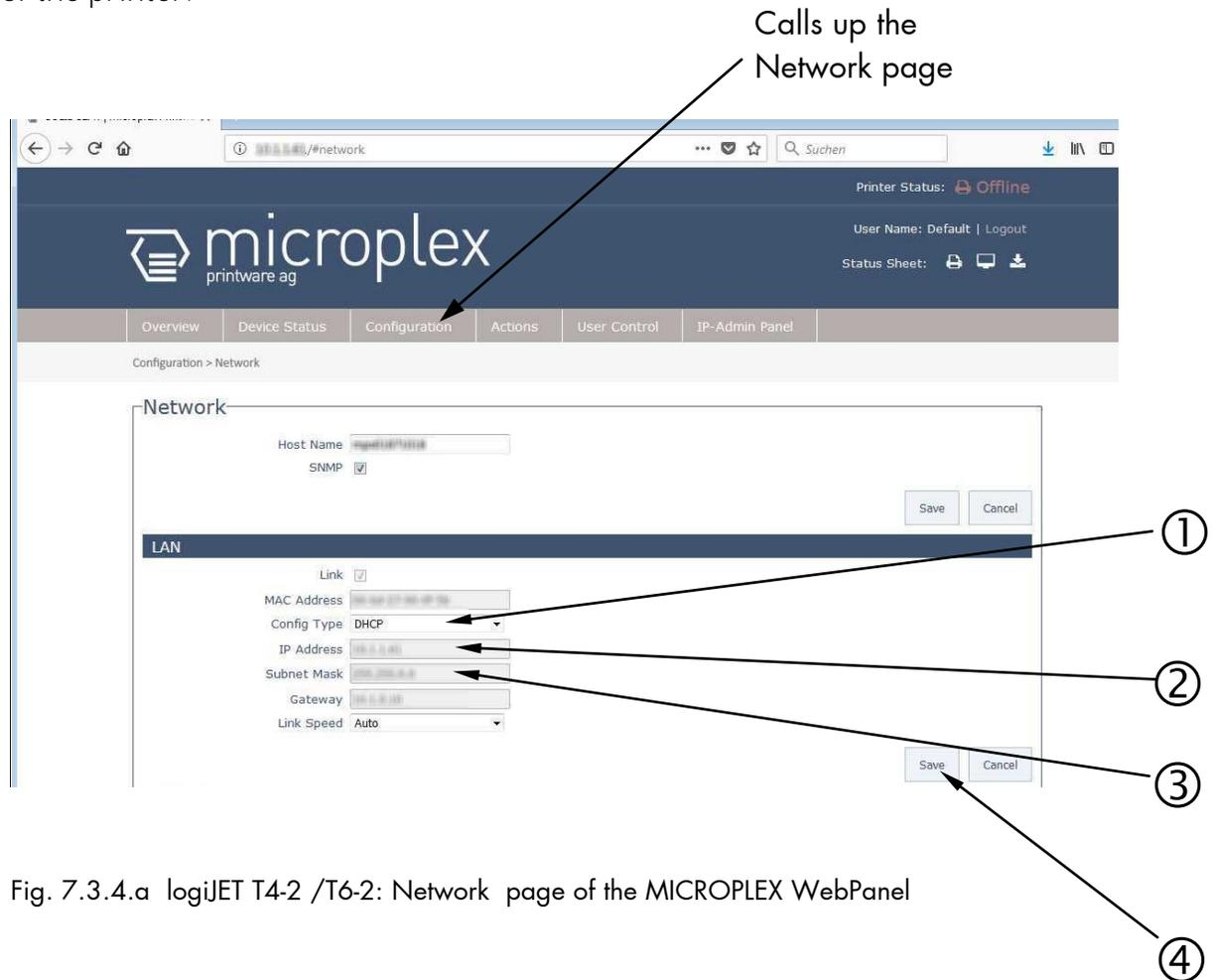
Fig. 7.3.4.a logiJET T4-2 /T6-2: Network page of the MICROPLEX WebPanel
