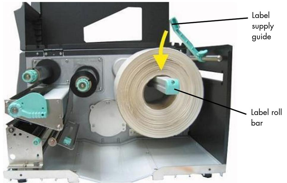
Fig. 5.2.1.e Inserting the media roll
