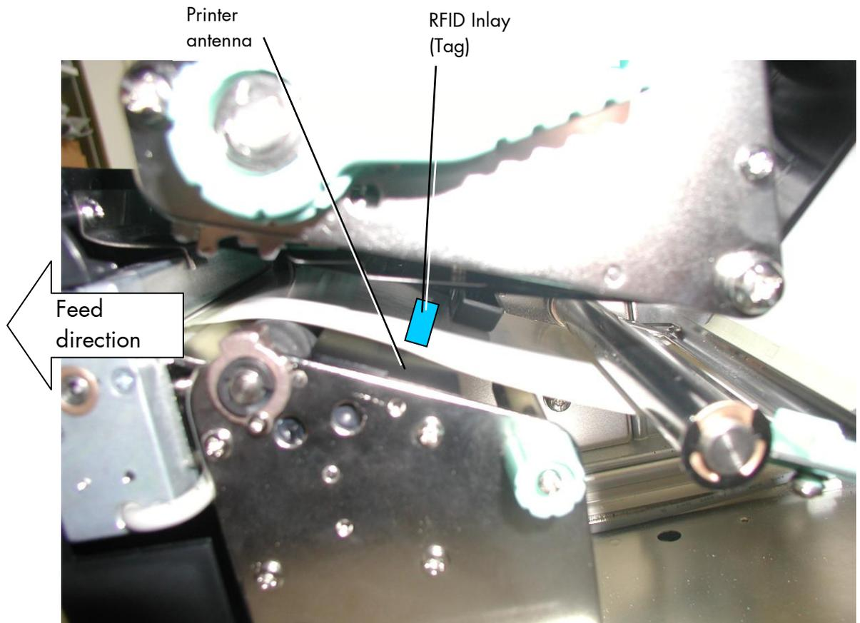
Fig. 10.2.3.b View into the printer: Check the position of the RFID Inlay above the printer antenna
