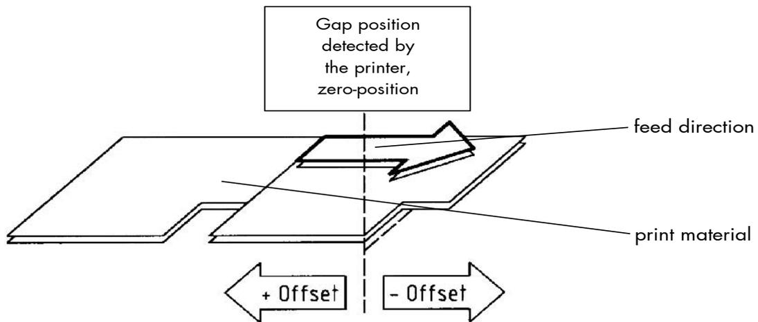
Fig. 9.4.a Adjusting the Zero Position of the Material Transport
