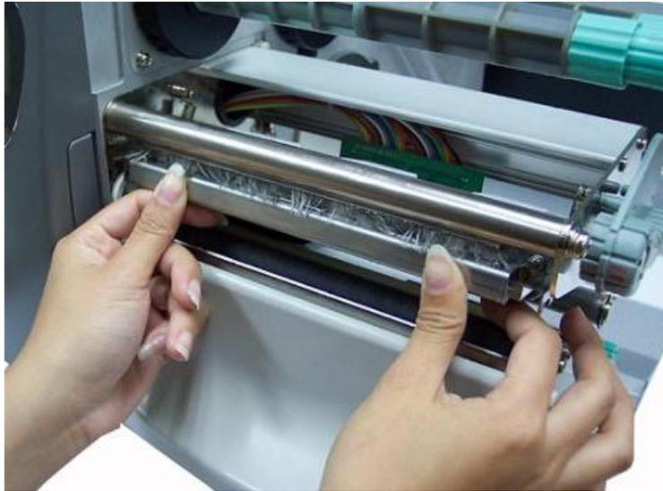
Fig. 11.2.1.f Inserting the printhead into its carriage
