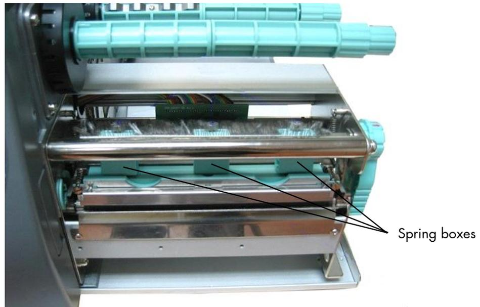
Fig. 5.4.a Printhead contact pressure: position of the spring boxes
