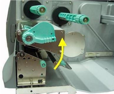
Fig. 11.2.1.a Pull the printhead pressure lever out and swivel it upward (counterclockwise).
