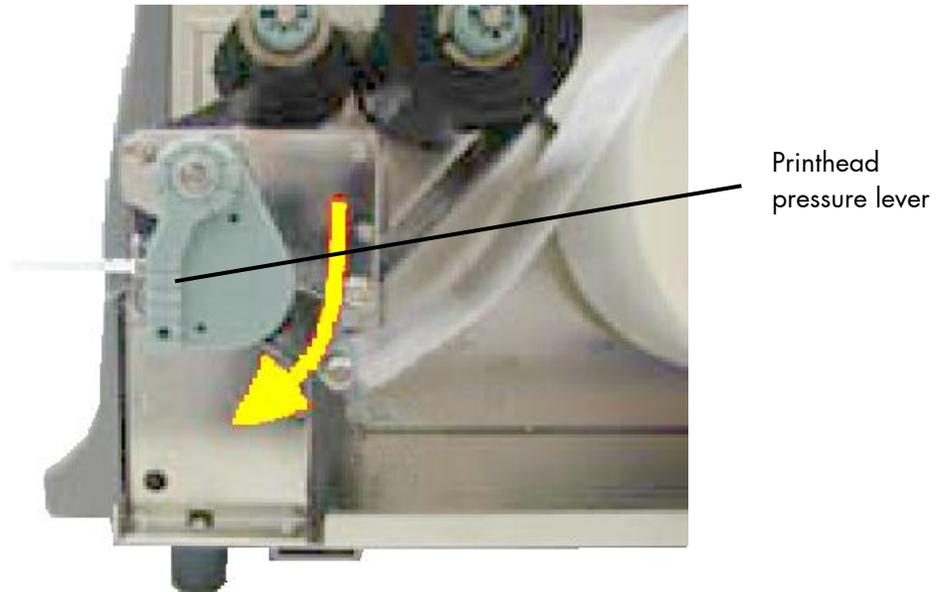
Fig. 5.3.1.f Locking the pressure lever
