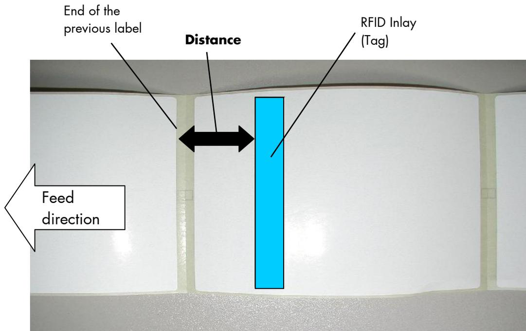
Fig. 10.2.3.a Measuring the transponder position
