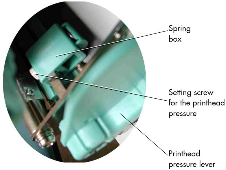
Fig. 5.4.d Detailed picture of a spring box
