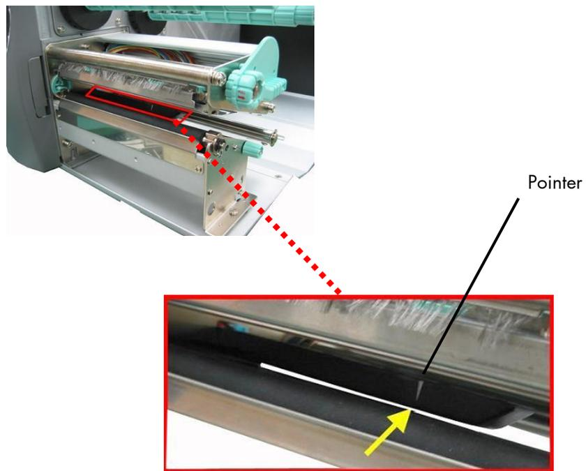
Fig. 9.3.1.e The pointer indicates the sensor position
