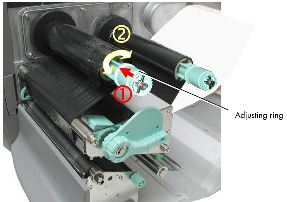
Fig. 5.3.2.a Adjusting the ribbon tension at the ribbon rewind shaft
