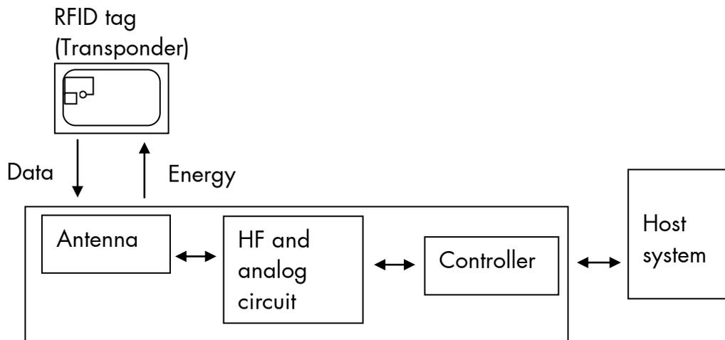
Fig. 1.2.a Block diagram: High Frequency Identification technology (RFID)
