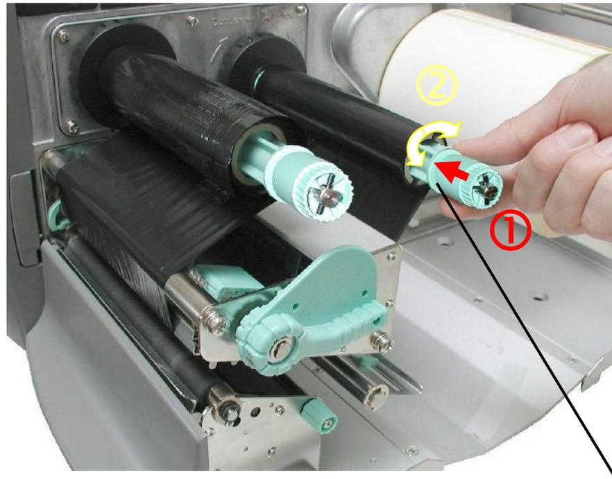
Fig. 5.3.2.a Adjusting the ribbon tension at the ribbon supply shaft
