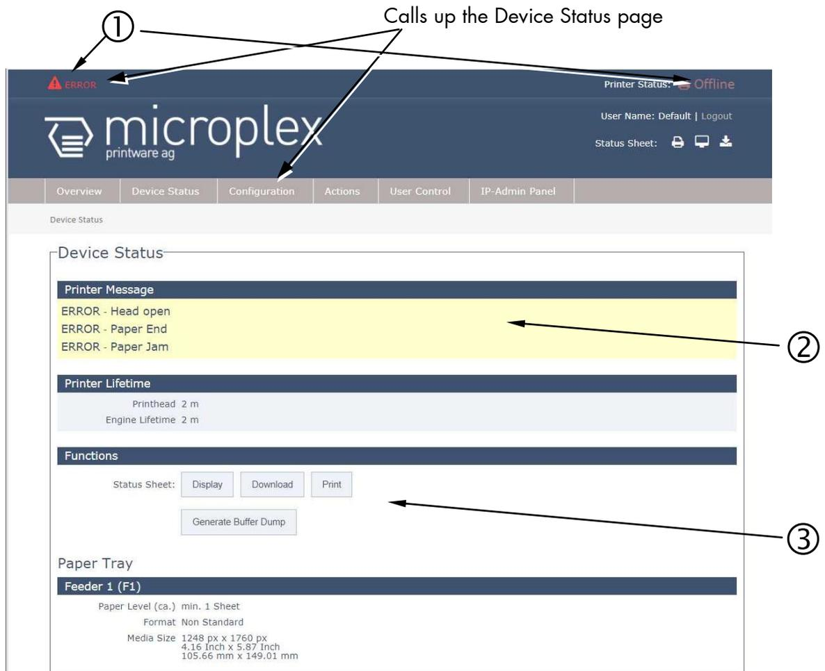
Fig. 7.3.5.a logiJET T4-2 /T6-2: Device Status page of the MICROPLEX WebPanel
