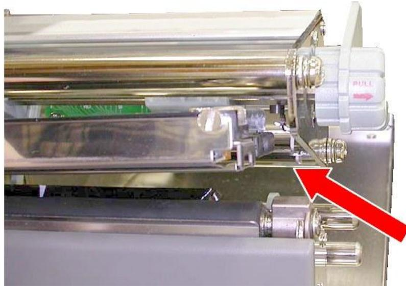
Fig. 11.2.1.d Insert the printhead into the side guides
