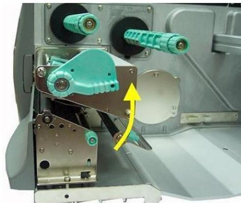
Fig. 5.3.1.a Swivel the printhead pressure lever upward (counterclockwise).
