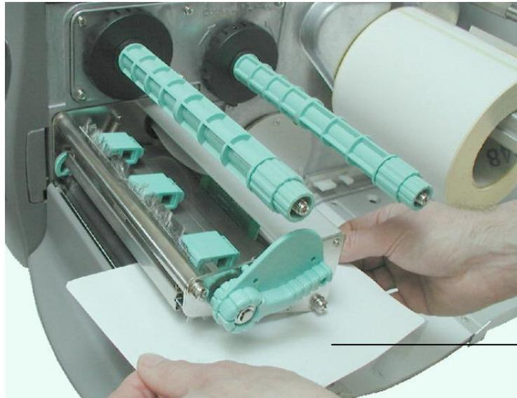
Fig. 11.1.2.b Cleaning the printhead using a cleaning strip
