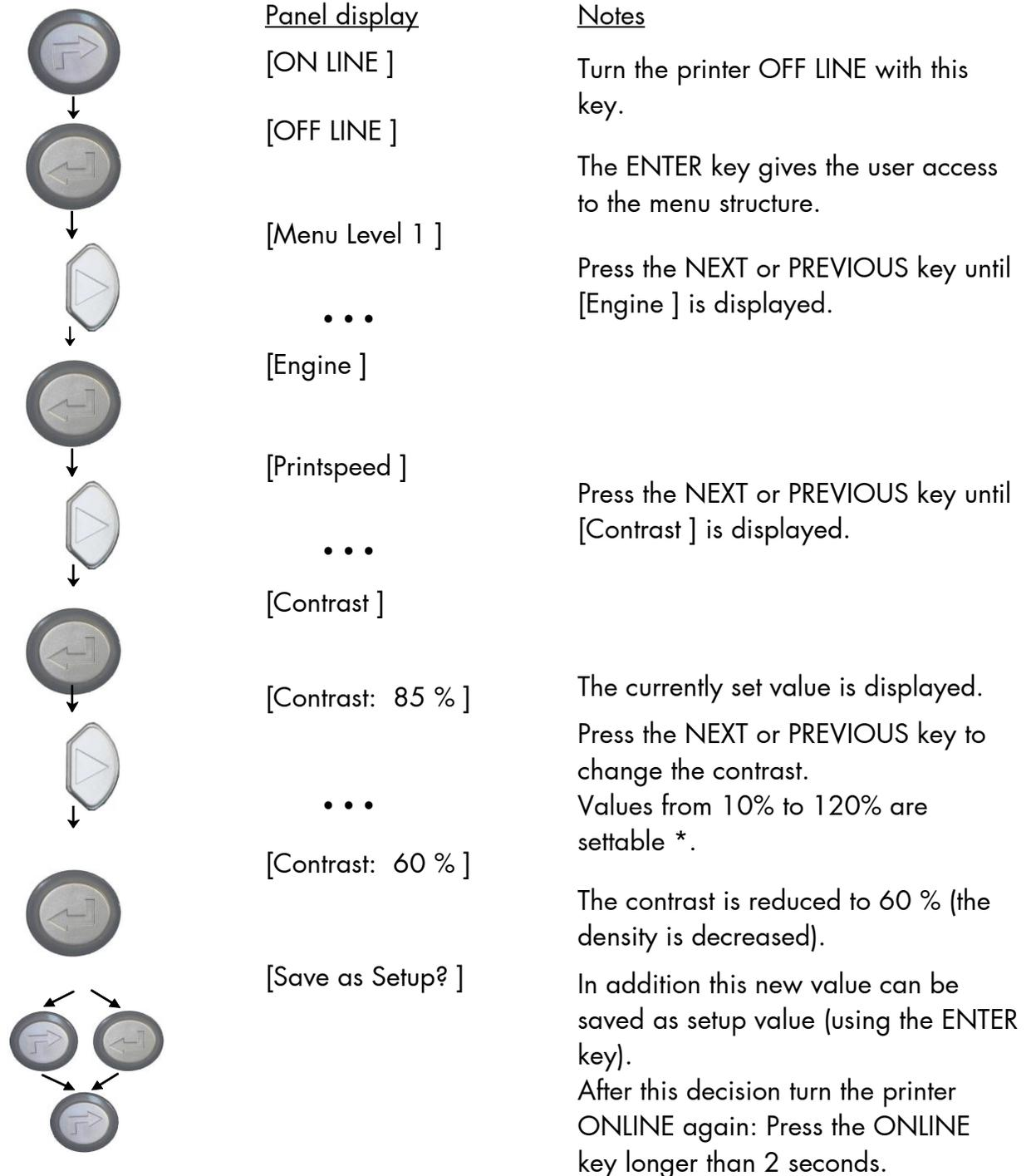
**\* Note:** Please consider that using high contrast values (more than 100%) can result in a reduced lifetime of the printhead.
