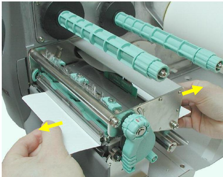
Fig.11.1.2.c Moving the cleaning strip in both directions
