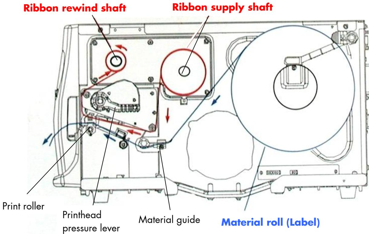
Fig. 5.1.a Winding directions of material and ribbon (here: ink inside the roll)
