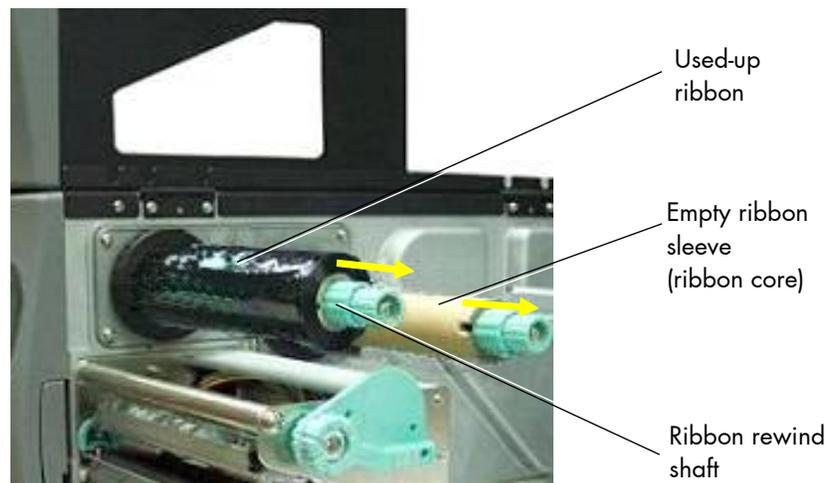
Fig. 5.3.3a Removing used-up ribbon
