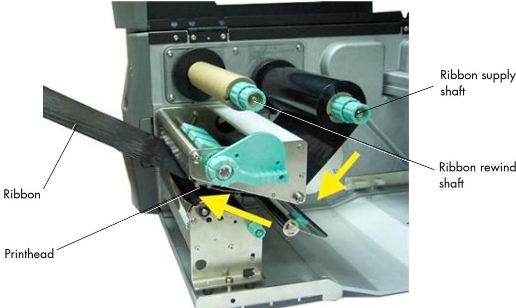
Fig. 5.3.1.d Feeding through the ribbon below the printhead
