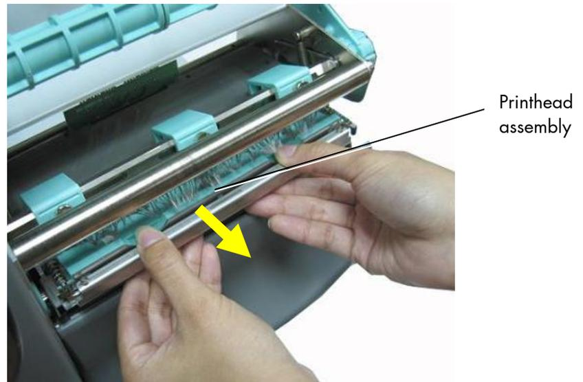
Fig. 11.2.1.b Gently pull the printhead a little bit towards you
