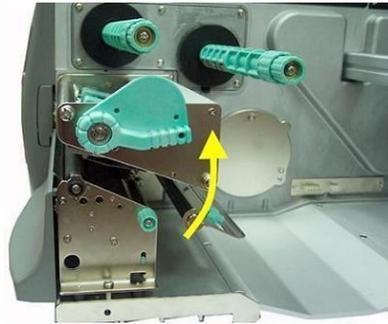
Fig. 5.4.b Swivel the printhead pressure lever upward (counterclockwise).
