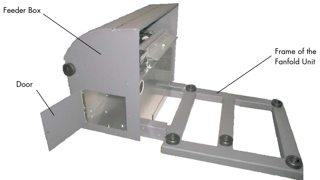
Fig. 3.2.a Setting the Feeder Box onto the Frame
