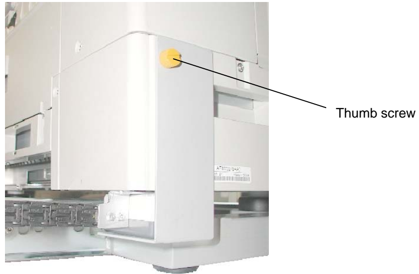
Fig. 3.4.e Connector and fixing bracket mounted to the printer
