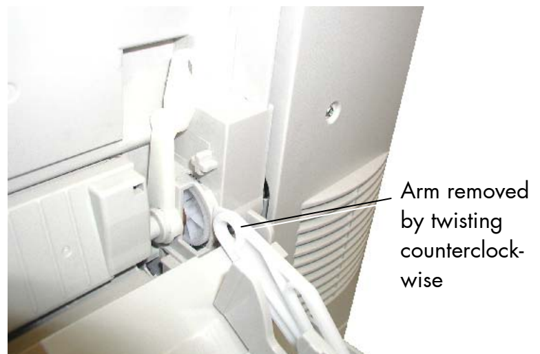
Fig. 2.2.1.f Right side: arm removed by twisting counterclockwise
