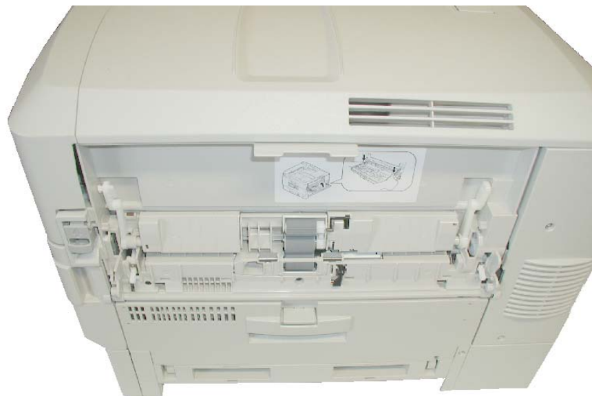
Fig. 2.2.1.n MPT removing completed
