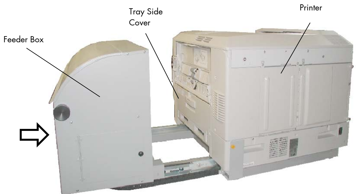
Fig. 7.a Moving the Fanfold Unit towards the printer
