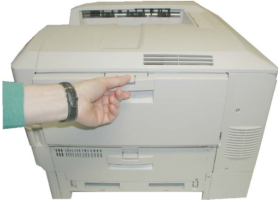
Fig. 2.2.1.a Opening the Multi-Purpose Tray (MPT)
