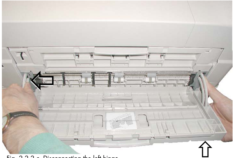
Fig. 2.2.2.c Disconnecting the left hinge
