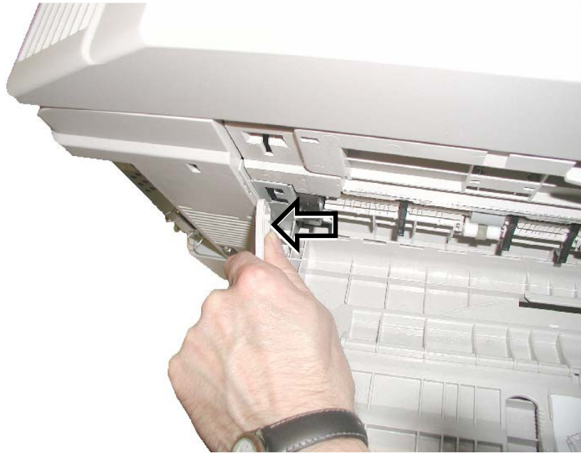
Fig. 2.2.2.d Detail: left side hinge disassembled
