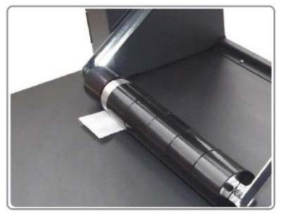
Insert a straightened paperclip into the hole on the side with the power switch and two LEDs. This will engage a button inside the rewinder. Keep the button pressed and turn on the device. The yellow LED will be flashing. Remove the clip.
